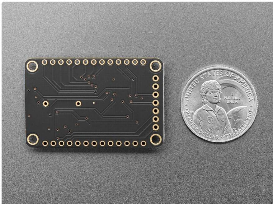
The IS31FL3731 is a nice little chip - it can use 2.7-5.5V power and logic so it's flexible for use with any microcontroller. You can set the address so up to 4 matrices can
