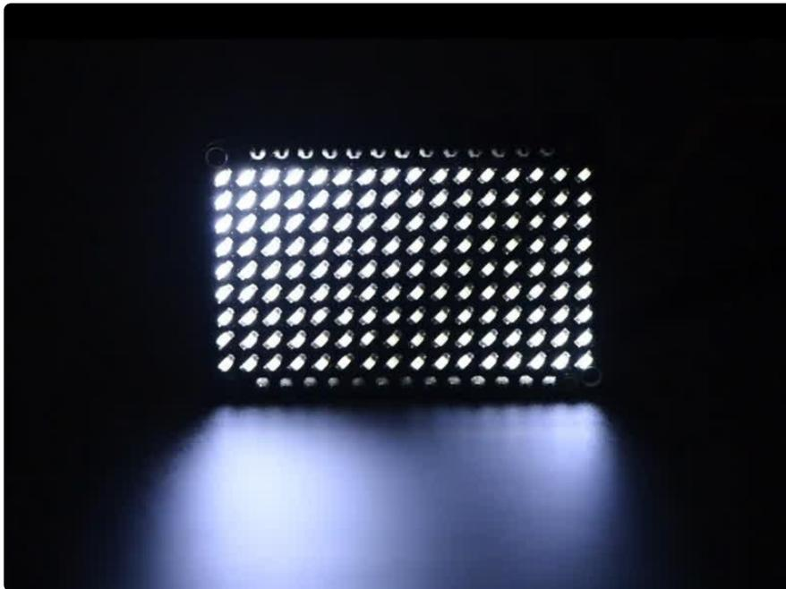
Pick up a driver board and your favorite color LEDs to match. You'll need to do some basic soldering to attach the driver backpack and matrix together, and run wires to your microcontroller, but its not too hard. Then install our Arduino or CircuitPython libraries to get some LEDs blinking immediately. Our library is Adafruit\_GFX compatible so you can draw lines, circles, text, and small bitmaps if you want more graphics control.
