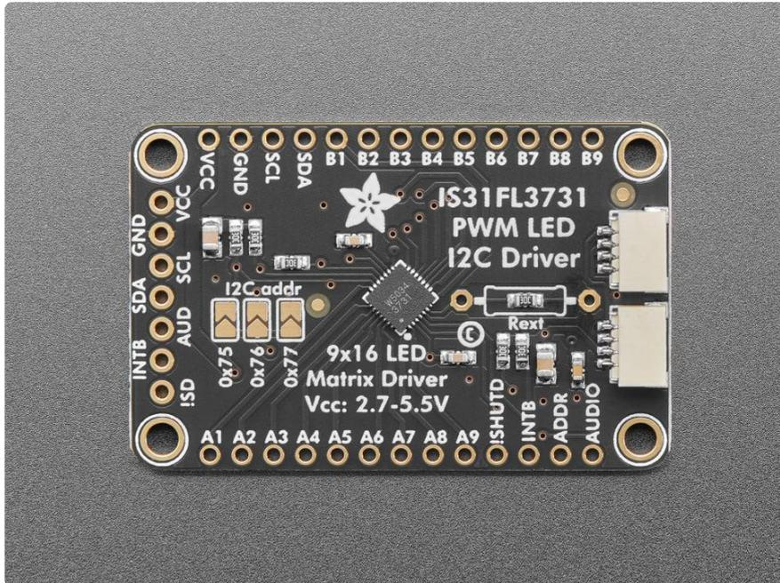
The IS31FL3731 will let you get back to that classic LED matrix look, with a nice upgrade! This I2C LED driver chip has the ability to PWM each individual LED in a 16x9 grid so you can have beautiful LED lighting effects, without a lot of pin twiddling. Simply tell the chip which LED on the grid you want lit, and what brightness and it's all taken care of for you.
