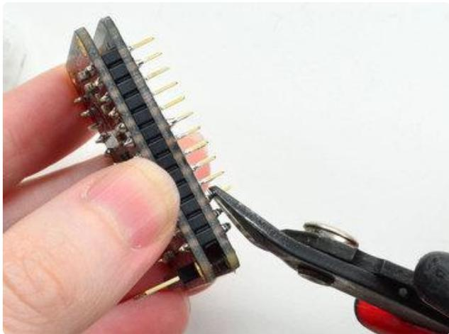
Watch out for flying header bits. Wear eye protection and be careful!
