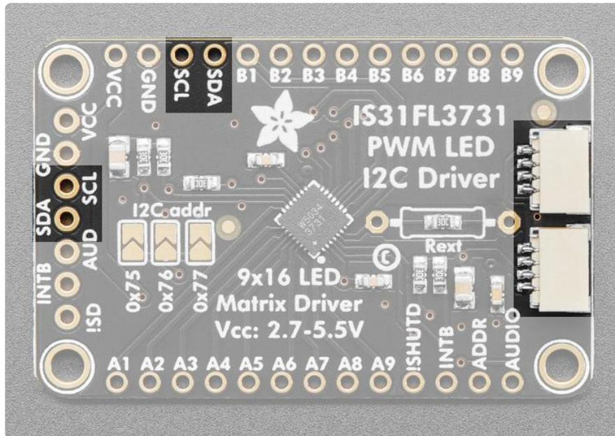
This chip uses I2C for control, it does not use clock stretching or repeated start. There are built in 20K pullups to VCC. You can run it as fast as 400KHz clock speed, but you may need to add additional 2K pullups from SDA and SCL up to VCC for higher speeds
