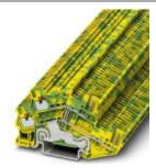
Protective conductor double-level terminal block, Cross section: 0.14 mm² - 1.5 mm², AWG: 26 - 14, Connection type: Push-in connection, Width: 3.5 mm, Color: green-yellow, Mounting type: NS 35/7,5, NS 35/15
