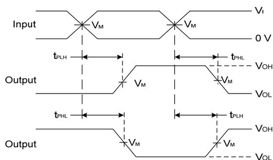
**Voltage Waveform Propagation Delay Times
