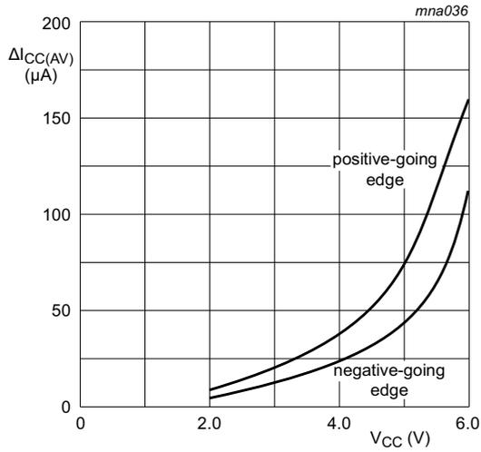
**Fig 14. Average additional I<sub>CC</sub> for 74AHC1G14 Schmitt trigger devices; linear change of V<sub>I</sub> between 0.1V<sub>CC</sub> to 0.9V<sub>CC</sub>**
