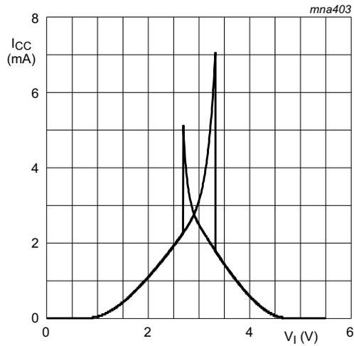
**Fig 11. Typical 74AHC1G14 transfer characteristics;**
