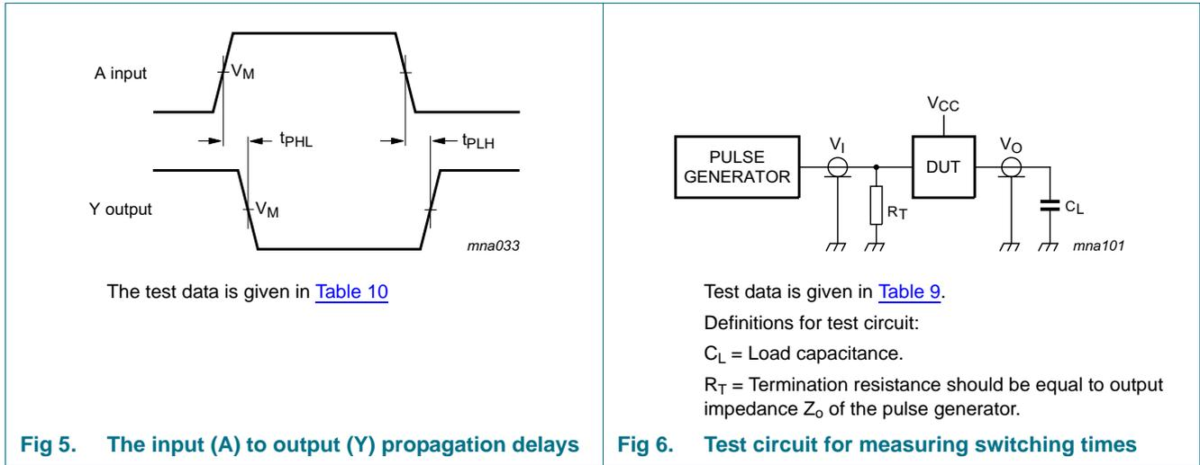
Fig 5. The input (A) to output (Y) propagation delays
