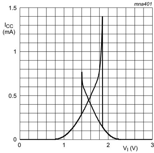
**Fig 9. Typical 74AHC1G14 transfer characteristics;**
