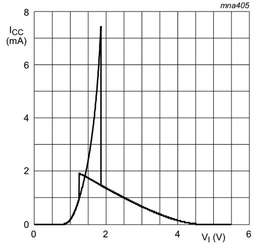
Fig 13. Typical 74AHCT1G14 transfer characteristics;  $V_{CC} = 5.5\text{ V}$
