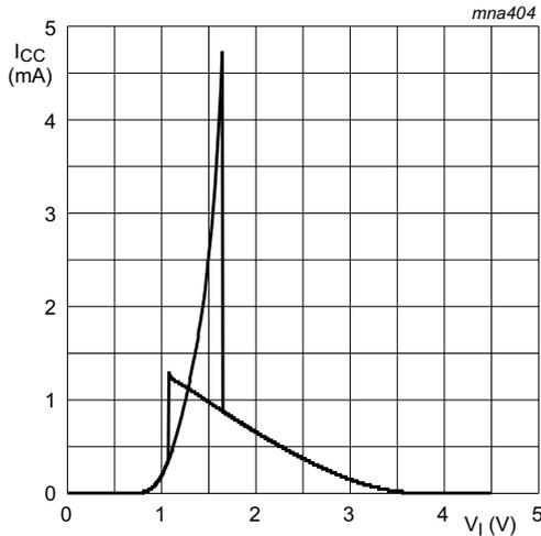
Fig 12. Typical 74AHCT1G14 transfer characteristics;  $V_{CC} = 4.5\text{ V}$
