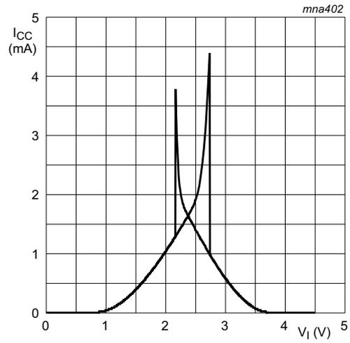
**Fig 10. Typical 74AHC1G14 transfer characteristics;**
