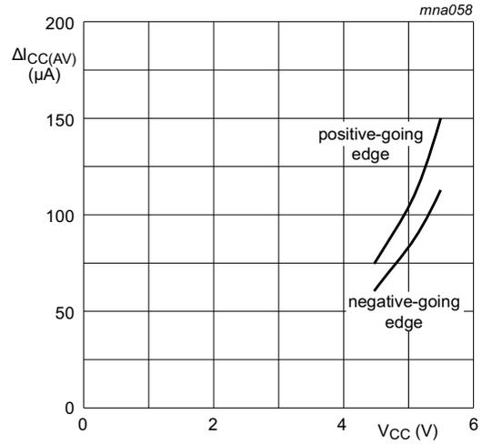
**Fig 15. Average additional I<sub>CC</sub> for 74AHCT1G14 Schmitt trigger devices; linear change of V<sub>I</sub> between 0.1V<sub>CC</sub> to 0.9V<sub>CC</sub>**
