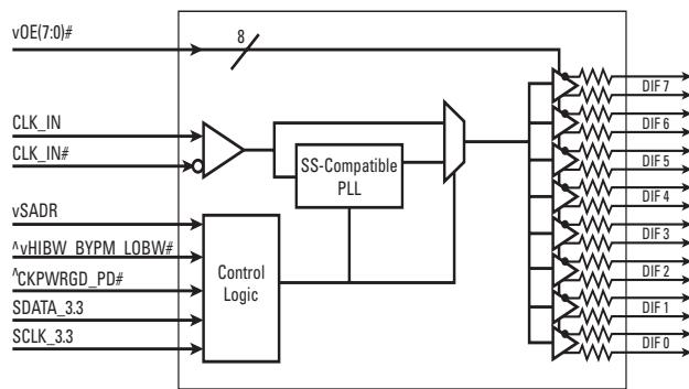
**9DBV0841 1.8V 8-output PCIe Gen 1/2/3 Zero Delay/Fan out Buffer with  $Z_o=100\ \Omega$**
