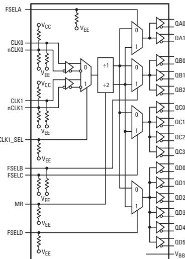
**8T33FS6222 - Low Voltage, 1:15 Differential PECL Clock Divider and Fanout Buffer**
