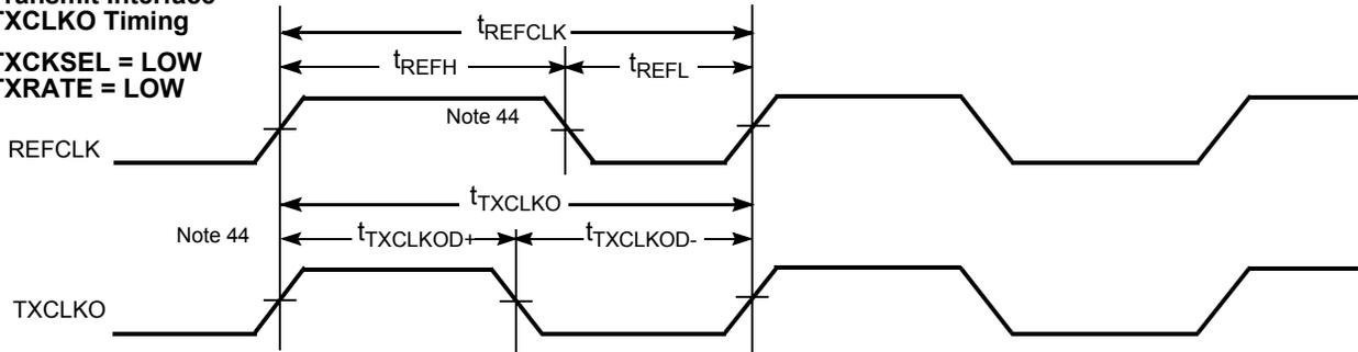
**Switching Waveforms for the CYP15G0201DXB HOTLink II Receiver**
