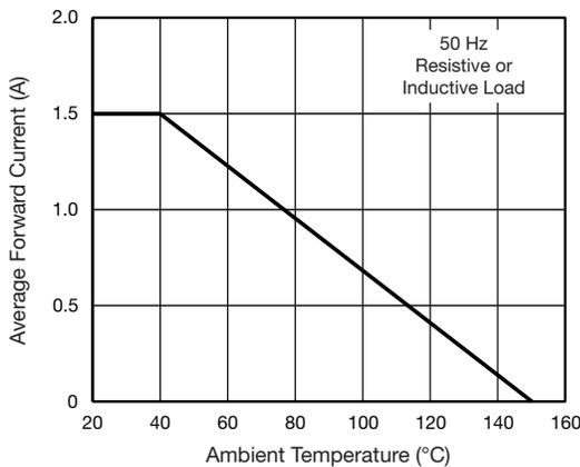
Fig. 1 - Forward Current Derating Curve Per Diode
