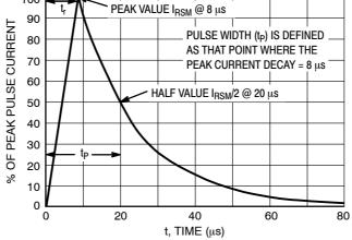
Figure 5. 8 x 20 μs Pulse Waveform
