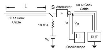
Figure 8. Simplified Schematic of a Typical TLP System
