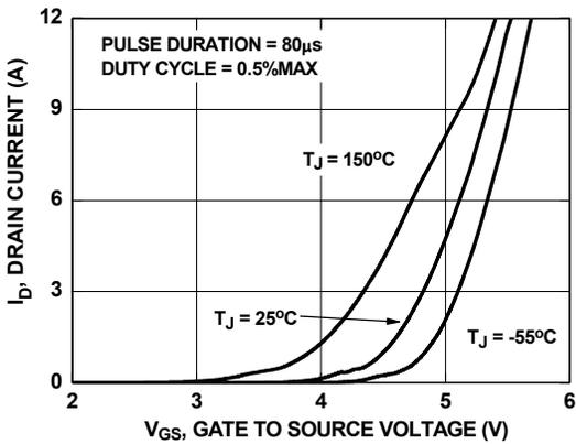
Figure 5. Transfer Characteristics
