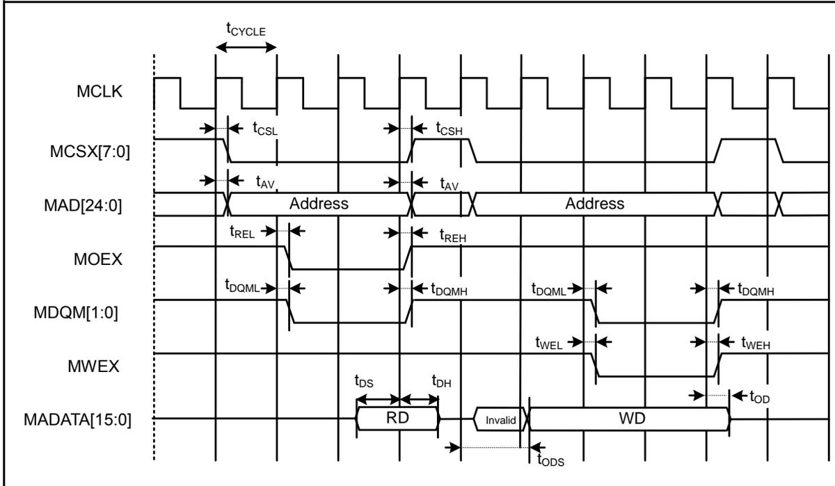
**Multiplexed Bus Access Asynchronous SRAM Mode**
