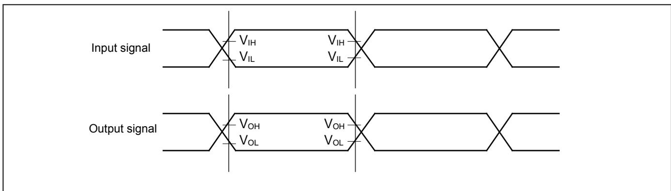
**Separate Bus Access Asynchronous SRAM Mode**
