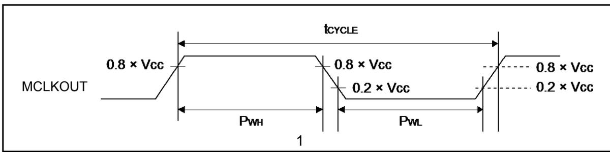
**External bus signal input/output characteristics**
