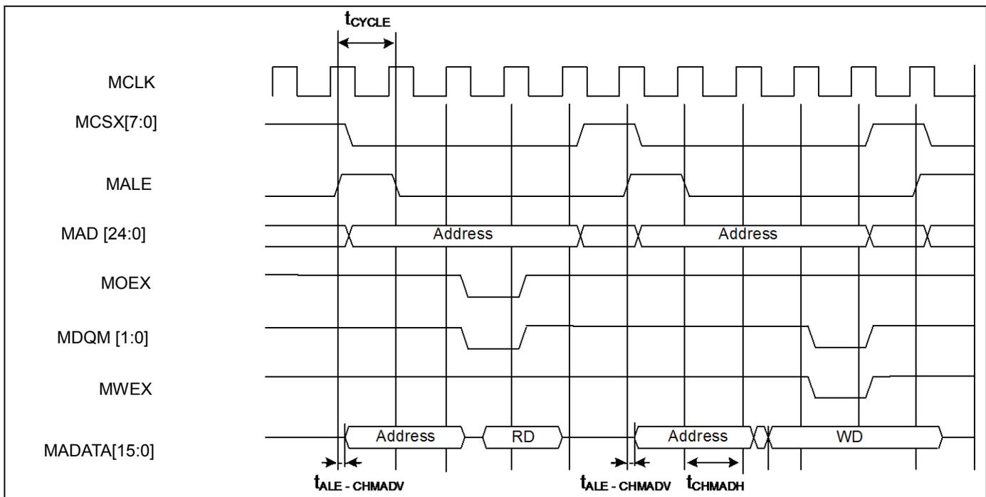
**Multiplexed Bus Access Synchronous SRAM Mode**
