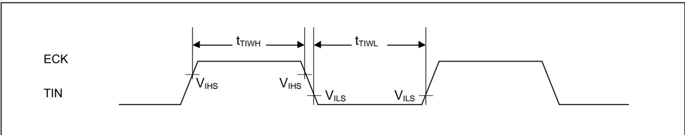
**Trigger input timing**
