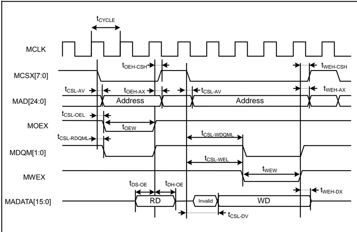
**Separate Bus Access Synchronous SRAM Mode**
