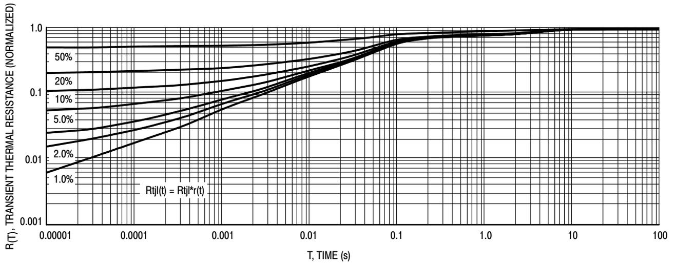
Figure 8. Thermal Response Junction to Lead
