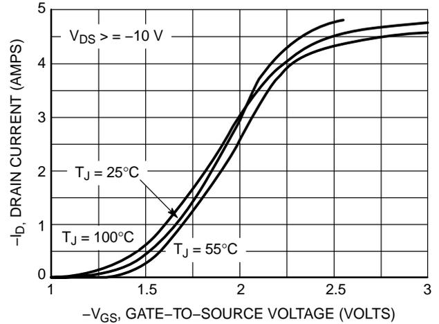
Figure 2. Transfer Characteristics
