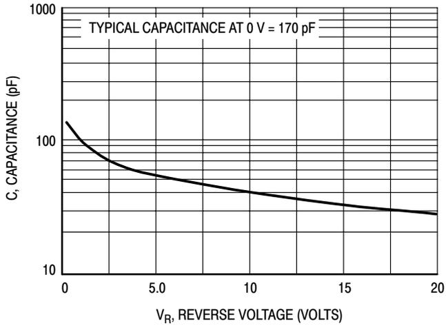
Figure 18. Typical Capacitance
