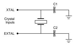
Figure 117. Circuit Configuration For Crystal
