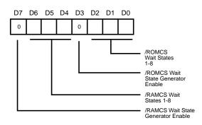
Figure 58. WSG Chip Select Register (Z180 MPU Read/Write, Address xxD8H)
