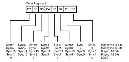
Figure 52. Write Register Bit Functions (Continued)
