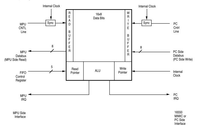
Figure 8. 16550 MIMIC Transmitter FIFO Block Diagram
