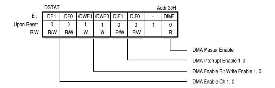
Figure 40. DMA Status Register
