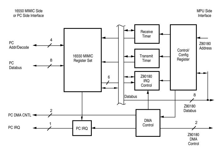
Figure 6. 16550 MIMIC Block Diagram
