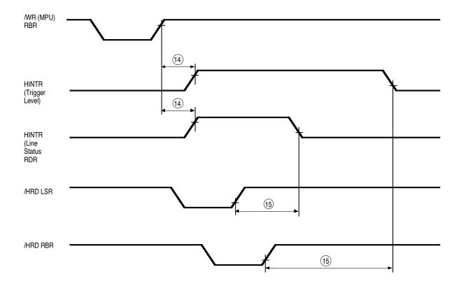
Figure 114. Interrupt Timing RCVR FIFO
