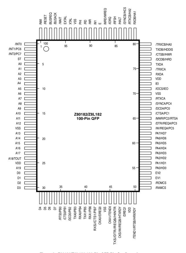
Figure 2. Z80182/Z8L182 100-Pin QFP Pin Configuration
