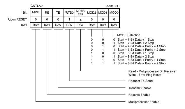
Figure 10a. ASCI Control Register A (Ch. 0)
