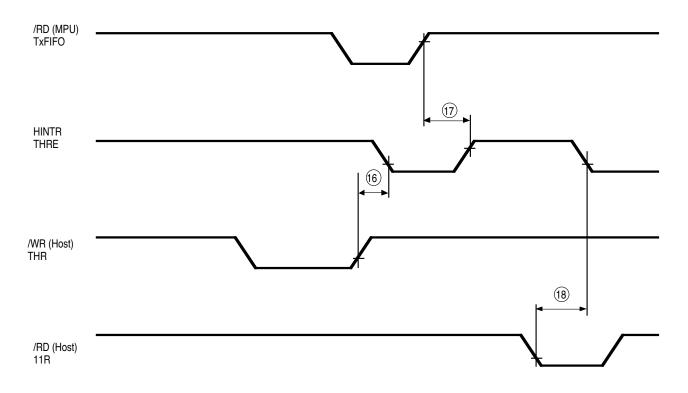
Figure 115. Interrupt Timing Transmitter FIFO
