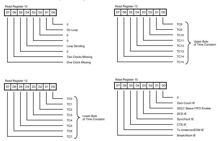
Figure 53. Read Register Bit Functions
