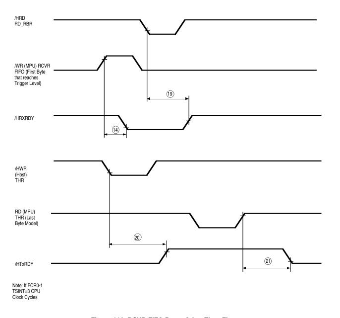
Figure 116 RCVR FIFO Bytes Other Than First
