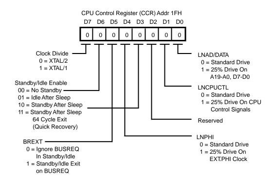
Figure 51. CPU Control Register
