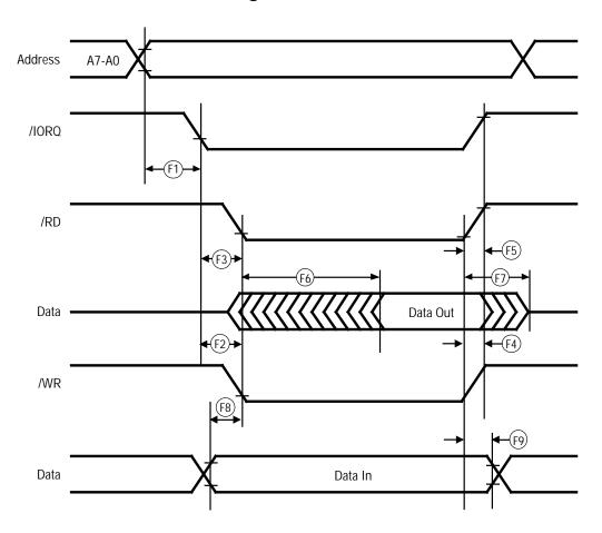
Figure 108. Read/Write External Bus Master Timing
