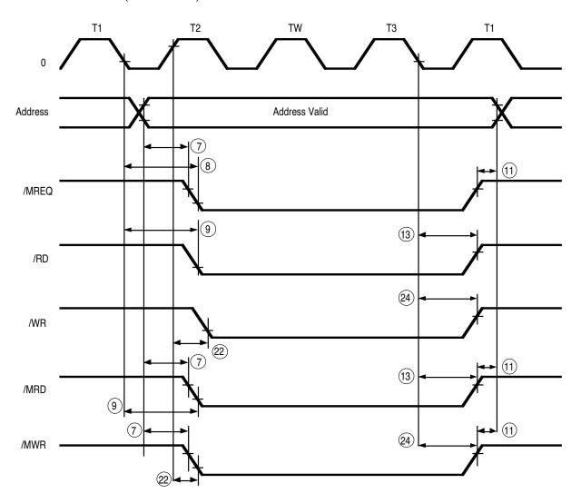
Figure 101. /MWR and /MRD Timing
