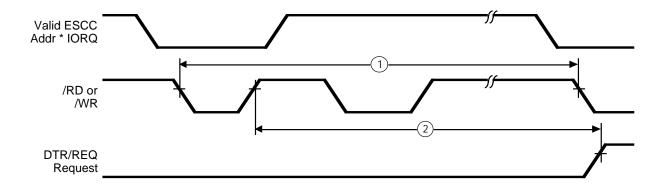
Figure 109. ESCC External Bus Master Timing
