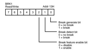
Figure 20. ASCI Break Control Register (Ch. 1)
