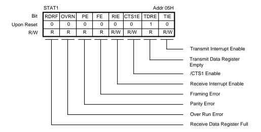
Figure 14. ASCI Status Register (Ch. 1)
