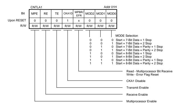
Figure 10b. ASCI Control Register A (Ch. 1)
