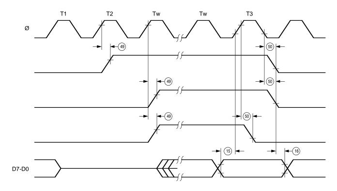
Figure 94. E Clock Timing (Memory Read/Write Cycle I/O Read/Write Cycle)
