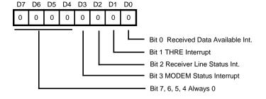
Figure 75. Interrupt Enable Register (PC Read/Write, Address 01H)
