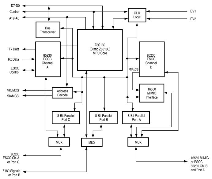
**Note**: Conventional use of the term "MPU side" refers to all interface through the Z180 MPU core and "PC side" refers to all interface through the 16550 MIMIC interface.
