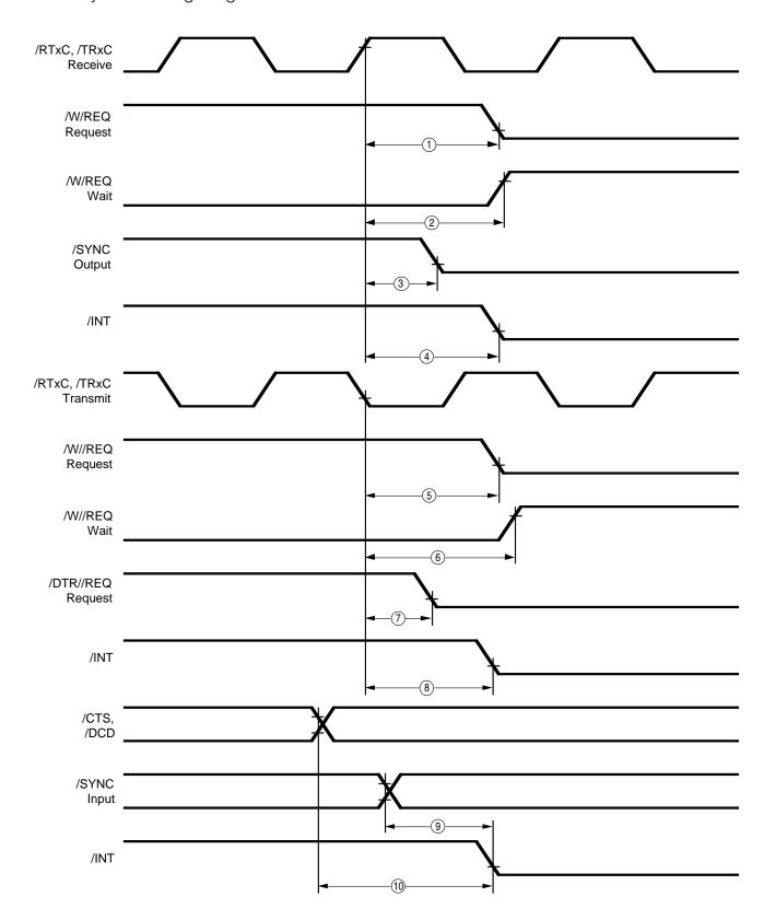
Figure 106. Z85230 System Timing
