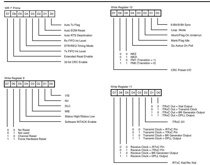
Figure 52. Write Register Bit Functions (Continued)
