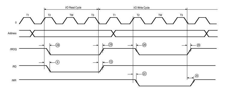
Figure 92. CPU Timing
