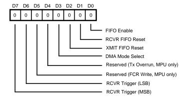
Figure 71. FIFO Control Register
