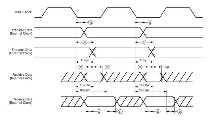
Figure 99. CSI/O Receive/Transmit Timing
