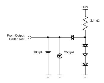
Figure 89. Test Load Diagram
