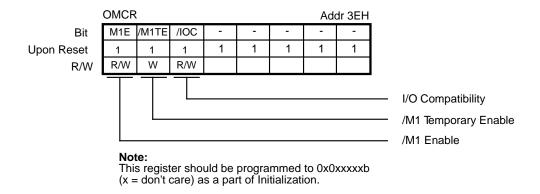
Figure 49. Operation Mode Control Register
