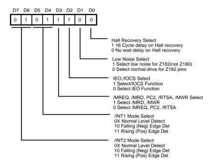
Figure 59. Interrupt Edge/Pin MUX Register
