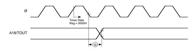
Figure 97. Timer Output Timing
