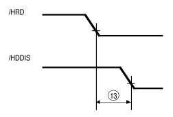
Figure 113. Driver Enable Timing
