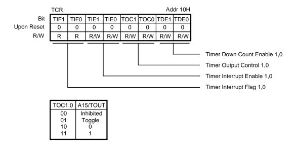
Figure 31. Timer Control Register
