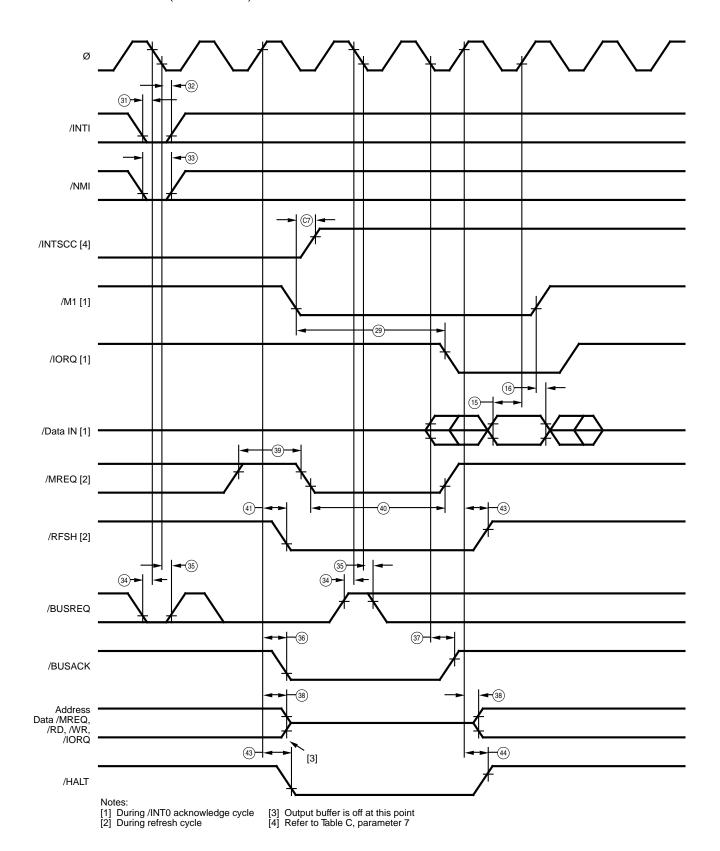
Figure 91. CPU Timing
