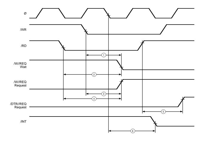
Figure 104. ESCC AC Parameter
