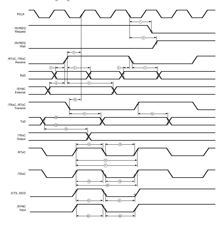
Figure 105. General Timing Diagram
