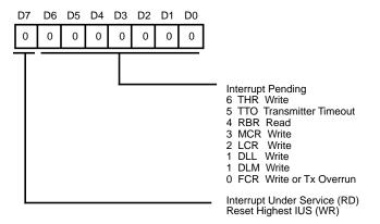
Figure 61. IUS/IP Register (Z180 MPU. Address xxFEH)
