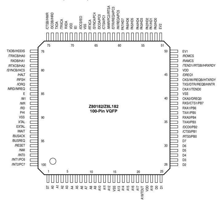
Figure 3. Z80182/Z8L182 100-Pin VQFP Pin Configuration
