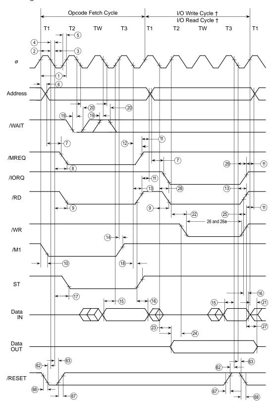
Figure 90. CPU Timing
