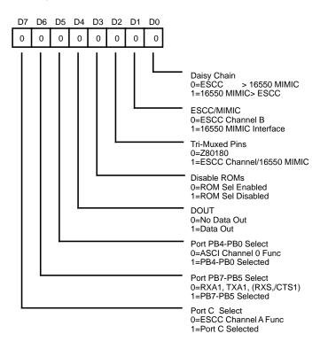
**Figure 54. System Configuration Register** (Z180 MPU Read/Write, Address xxEFH)
