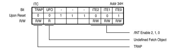
Figure 47. INT/TRAP Control Register
