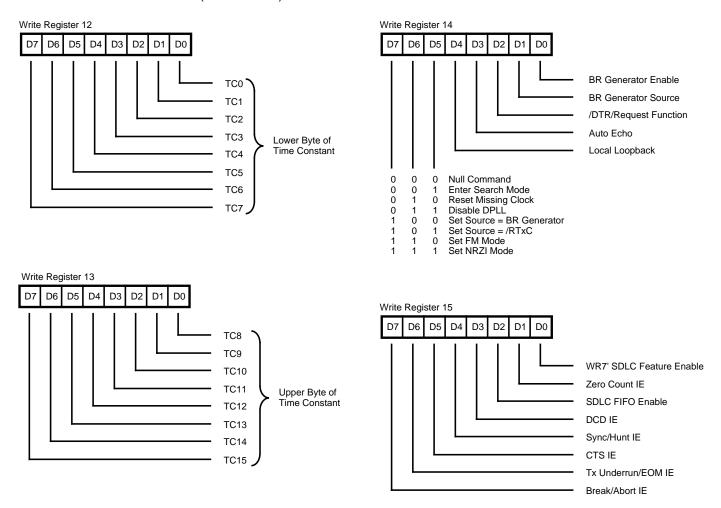
Figure 52. Write Register Bit Functions (Continued)
