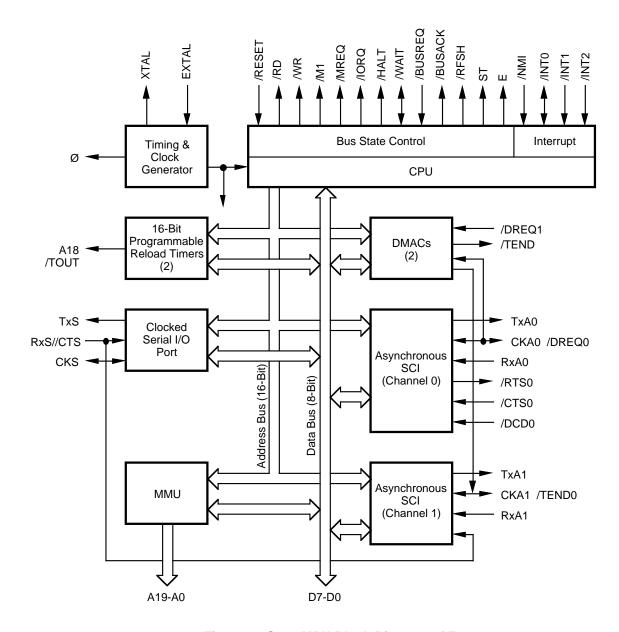
Figure 4. S180 MPU Block Diagram of Z182
