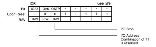
Figure 50. I/O Control Register
