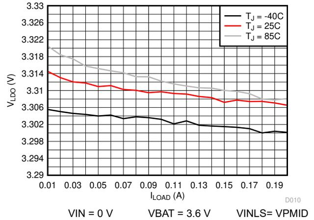
**Figure 8-8. LDO Load Regulation (VLDO = 3.3 V)**
