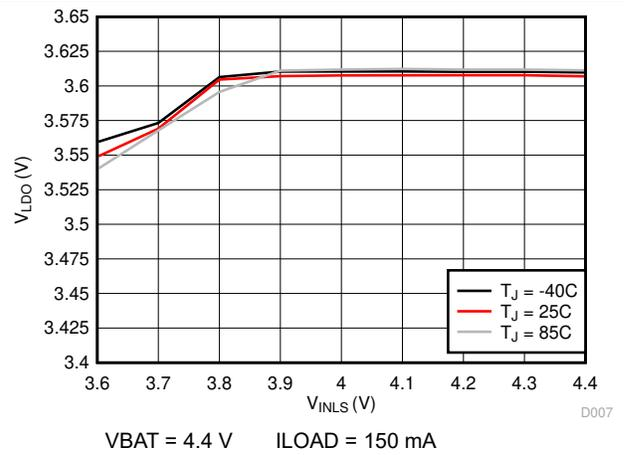
**Figure 8-12. LDO Line Regulation (VLDO = 3.6 V)**
