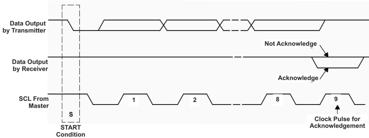
Figure 9-11. Acknowledge on the I<sup>2</sup>C Bus
