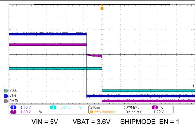
Figure 10-9. Ship Mode Entry on IN Supply Removal
