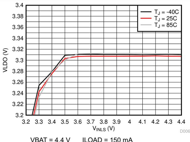
**Figure 8-11. LDO Line Regulation (VLDO = 3.3 V)**
