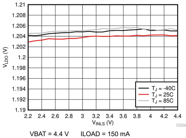
**Figure 8-9. LDO Line Regulation (VLDO = 1.2 V)**
