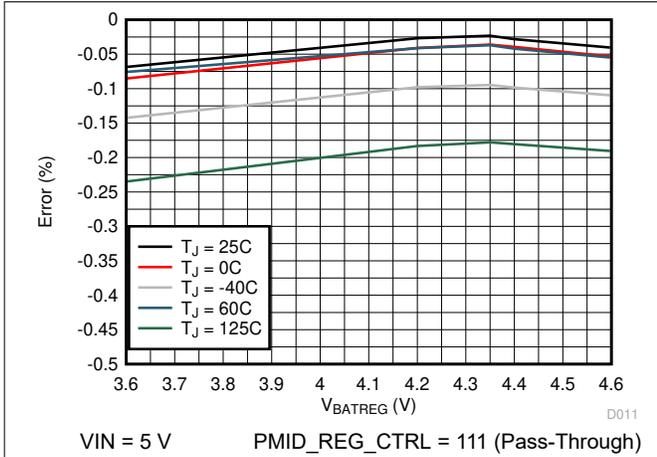
**Figure 8-1. Battery Regulation Voltage Accuracy vs. VBATREG Setting**
