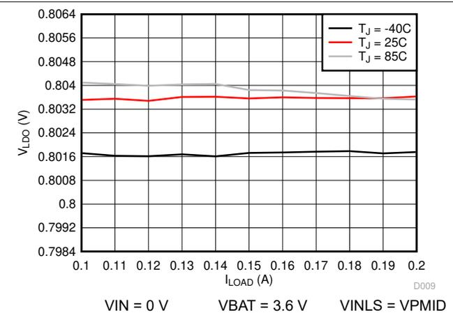
**Figure 8-6. LDO Load Regulation (VLDO = 0.8 V)**
