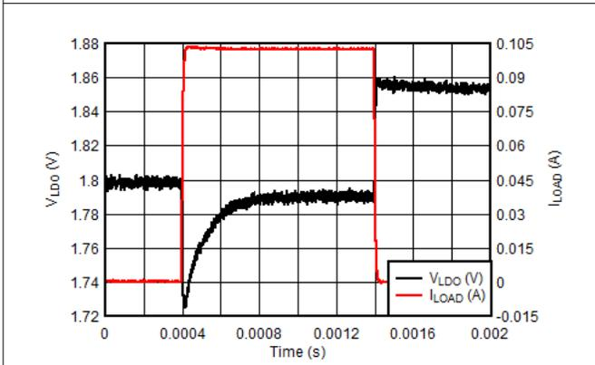
**Figure 10-18. LDO Load Transient - VLDO = 1.8V**
