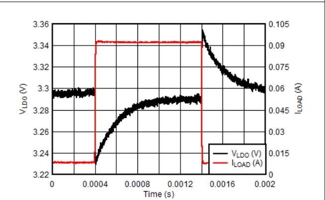
**Figure 10-19. LDO Load Transient - VLDO = 3.3V**
