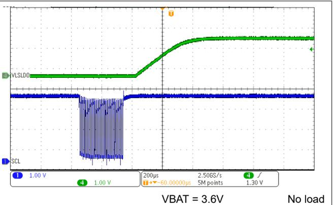
**Figure 10-15. LDO Enable Through I<sup>2</sup>C (EN\_LS\_LDO)**
