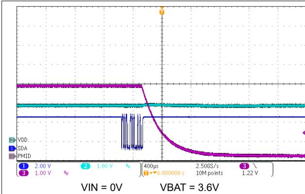
Figure 10-8. HW Reset Through I<sup>2</sup>C Command
