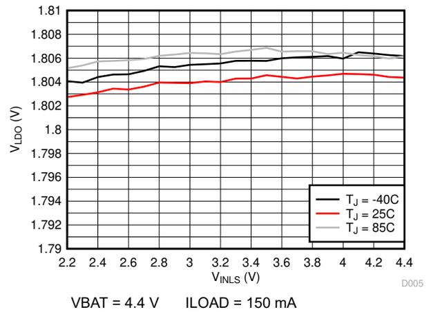
**Figure 8-10. LDO Line Regulation (VLDO = 1.8 V)**
