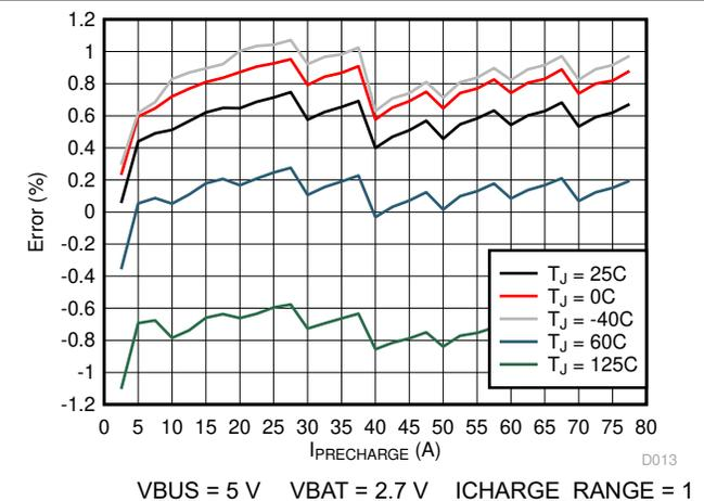
**Figure 8-4. Pre-Charge Current Accuracy vs. IPRECHARGE Setting (ICHARGE\_RANGE = 1)**
