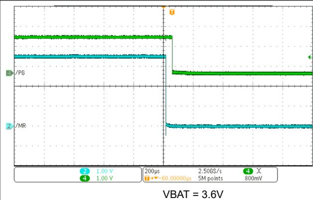
Figure 10-13.  $\overline{\text{PG}}$   $\overline{\text{MR}}$  Level Shift Function -  $\overline{\text{MR}}$  Falling
