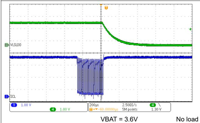
**Figure 10-16. LDO Disable Through I<sup>2</sup>C (EN\_LS\_LDO)**
