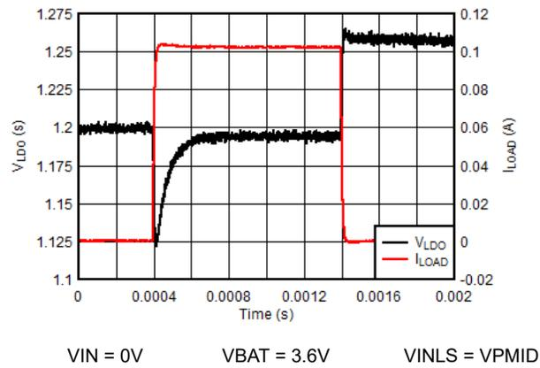
**Figure 10-20. LDO Load Transient - VLDO = 1.2V**
