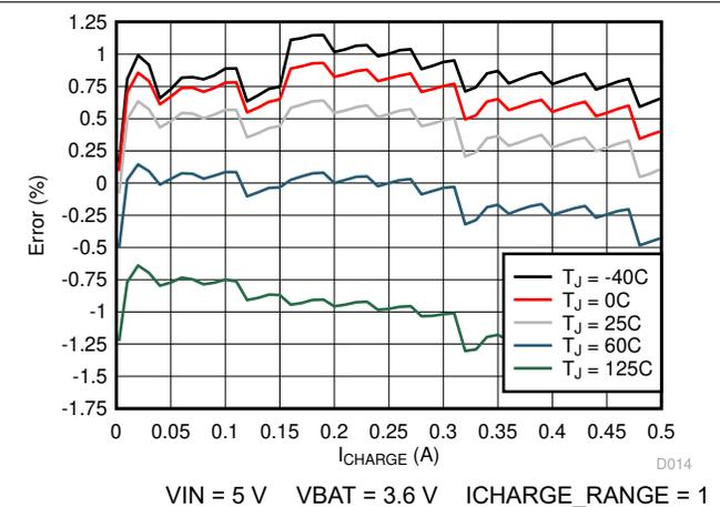
**Figure 8-2. Charge Current Accuracy vs. ICHARGE Setting**
