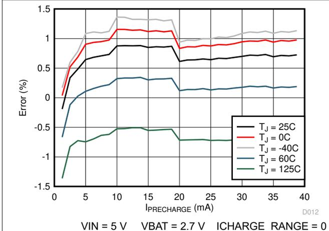
**Figure 8-3. Pre-Charge Current Accuracy vs. IPRECHARGE setting (ICHARGE\_RANGE = 0)**
