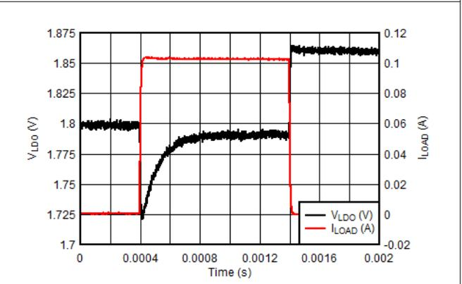
**Figure 10-17. LDO Load Transient - VLDO = 1.8V**
