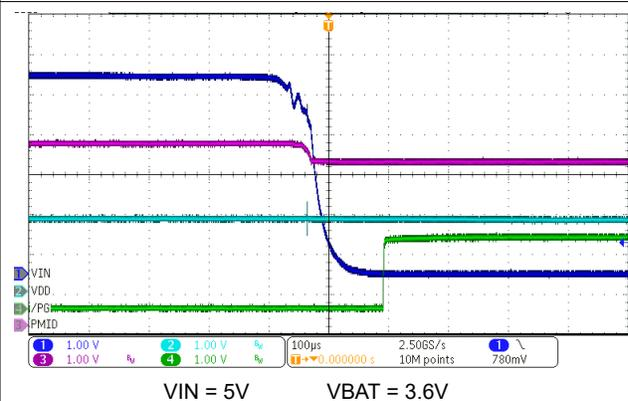
Figure 10-11.  $\overline{\text{PG}}$  Power Good Function - IN Supply Removal
