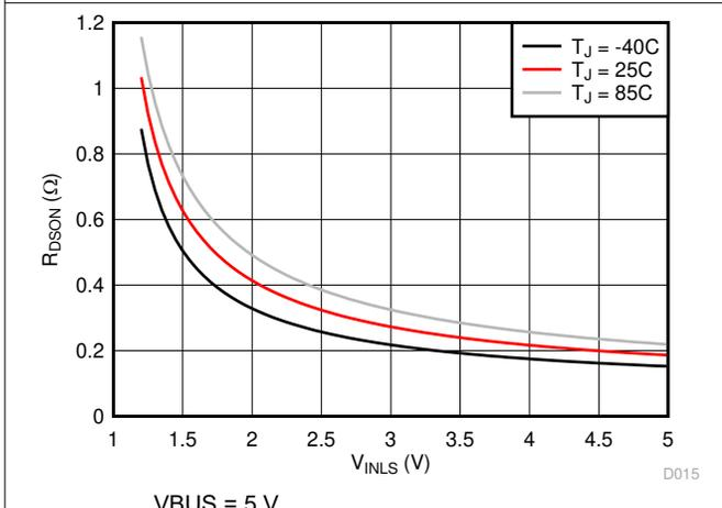
**Figure 8-5. LS/LDO Switch On Resistance vs. VINLS**
