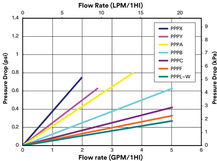
**Graph 1: Polypropylene Filter Flow Comparison**
