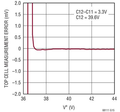
**Measurement Error vs Common Mode Voltage**
