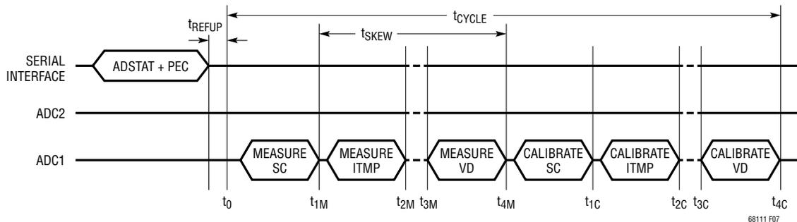
Figure 7. Timing for ADSTAT Command Measuring SC, ITMP, VA, VD
