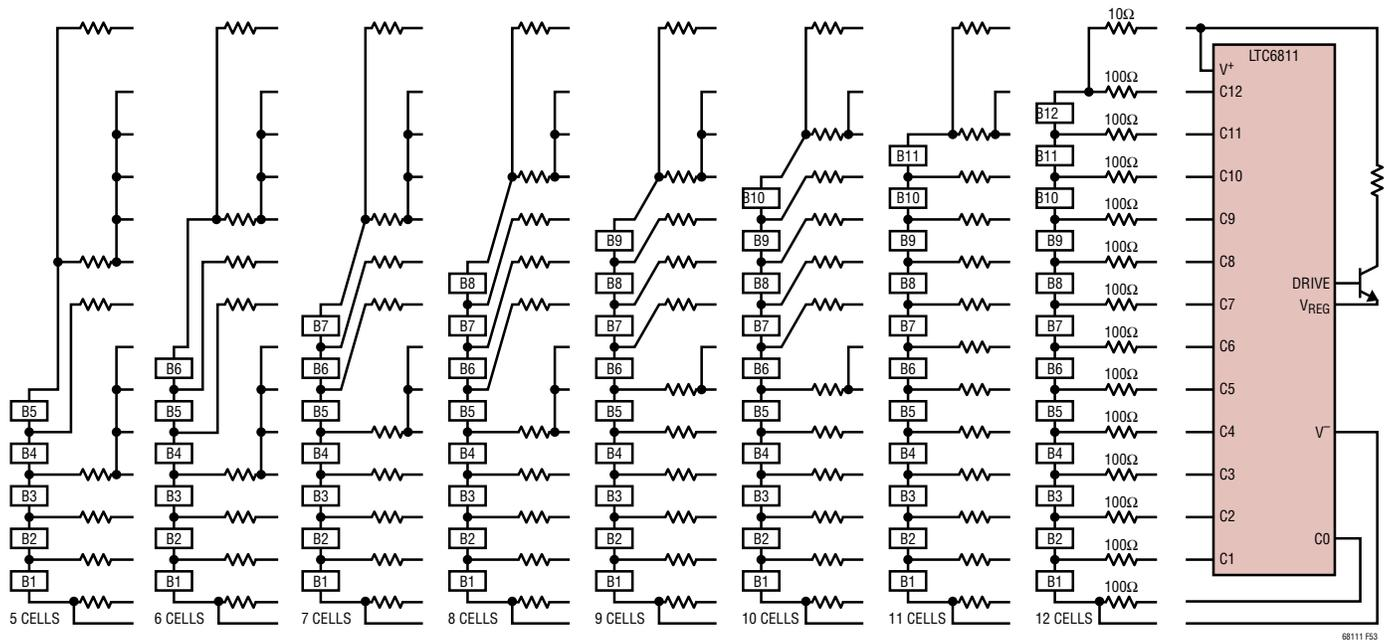
Figure 53. Cell Connection Schemes for 5 to 12 Cells
