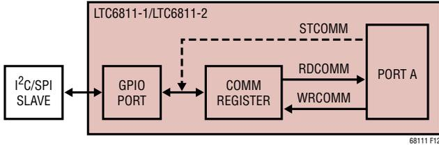
**Figure 12. LTC6811 I<sup>2</sup>C/SPI Master Using GPIOs**
