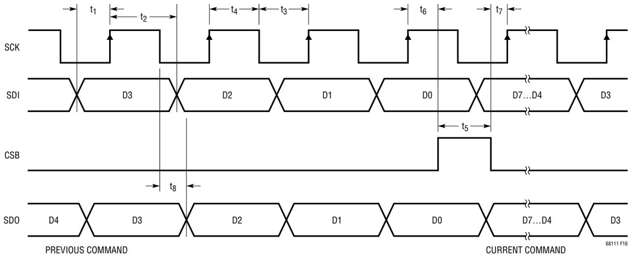
Figure 16. Timing Diagram of 4-Wire Serial Peripheral Interface
