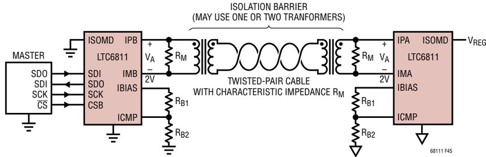
Figure 45. isoSPI Circuit
