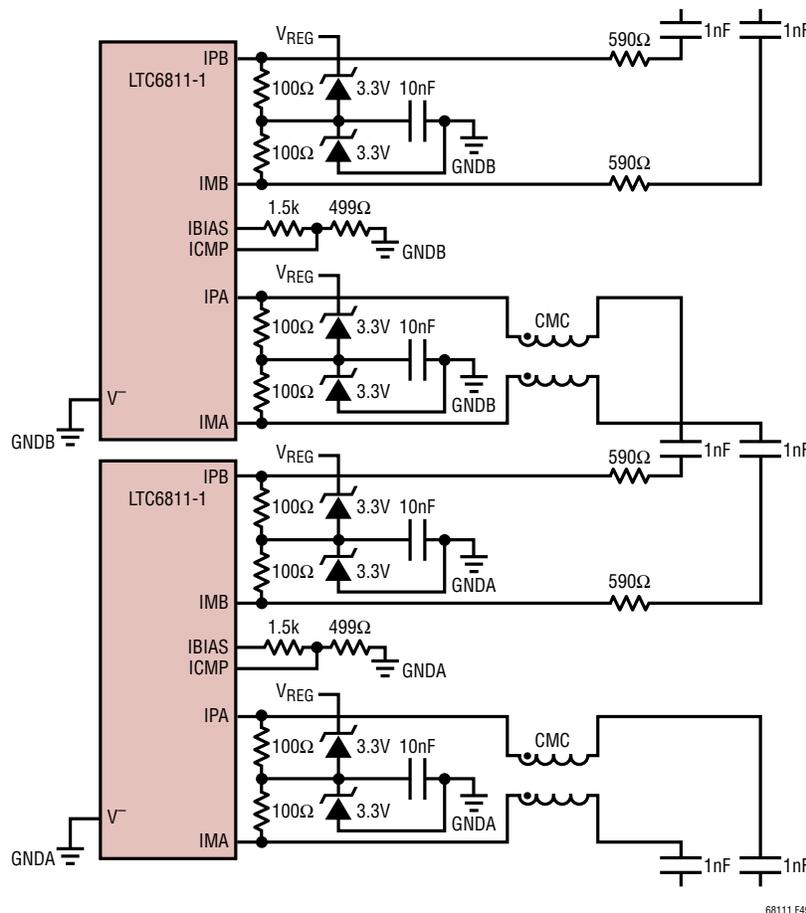
Figure 49. Capacitive Isolation Coupling for LTC6811-1s on the Same PCB
