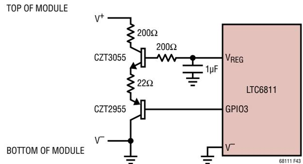
Figure 43. 200mA Module Balancer
