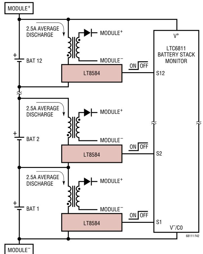
Figure 42. 12-Cell Battery Stack Module with Active Balancing
