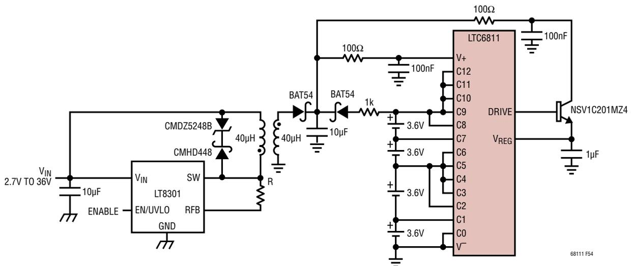
Figure 54. Powering the LTC6811 When Monitoring 4 Cells
