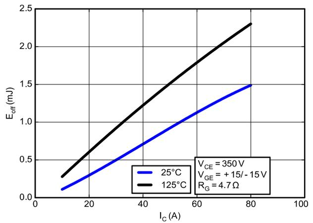
Figure 7. Typical Turn Off Loss vs. IC
