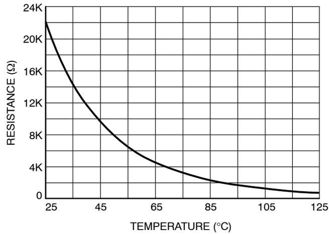
Figure 42. Thermistor Characteristics
