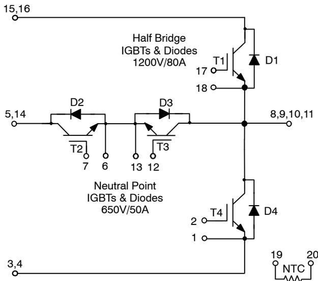
Figure 1. Schematic Diagram
