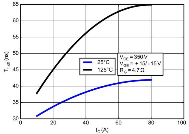
Figure 11. Typical Off Fall Times vs. IC
