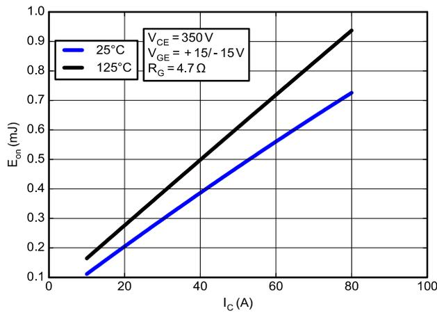
Figure 6. Typical Turn On Loss vs. IC
