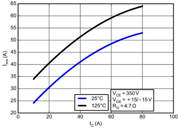
Figure 14. Typical Reverse Recovery Peak Current vs.  $I_C$
