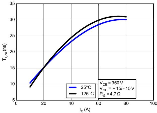
Figure 10. Typical On Rise Times vs. IC
