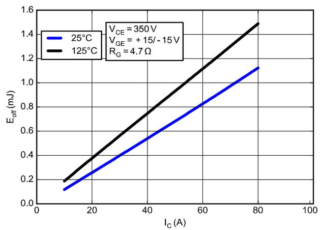
Figure 27. Typical Turn Off Loss vs. IC
