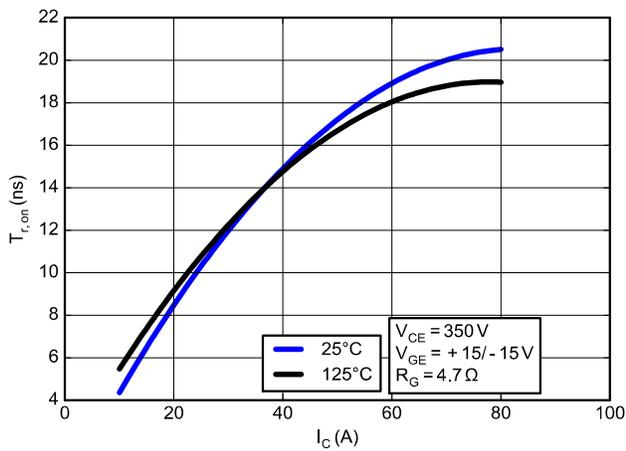
Figure 30. Typical On Rise Times vs. IC
