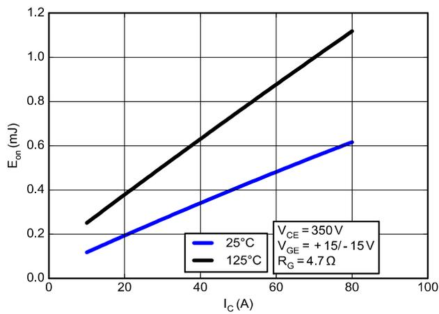
Figure 26. Typical Turn On Loss vs. IC
