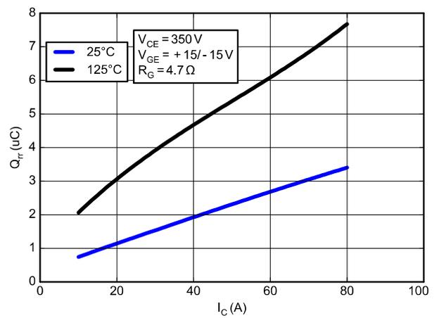
Figure 33. Typical Reverse Recovery Charge vs. IC
