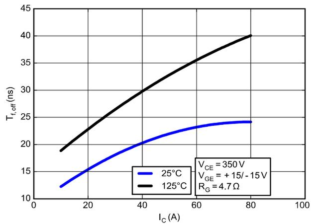
Figure 31. Typical Off Fall Times vs. IC
