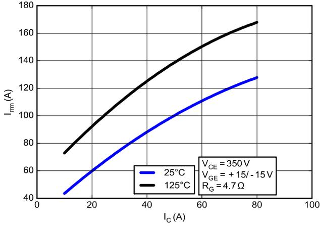
Figure 34. Typical Reverse Recovery Peak Current vs.  $I_C$
