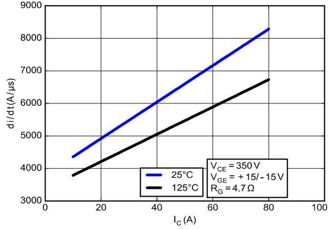
Figure 35. Typical Diode Current Slope vs.  $I_C$
