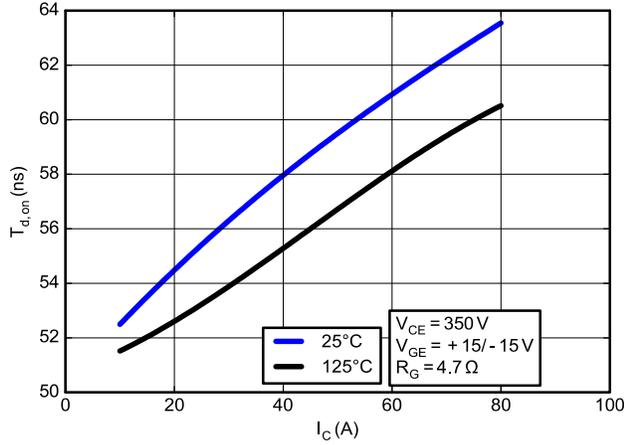
Figure 8. Typical On Switching Times vs. IC
