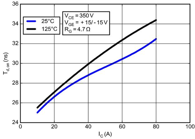
Figure 28. Typical On Switching Times vs. IC
