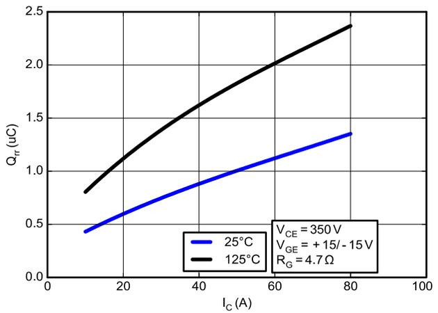
Figure 13. Typical Reverse Recovery Charge vs. IC
