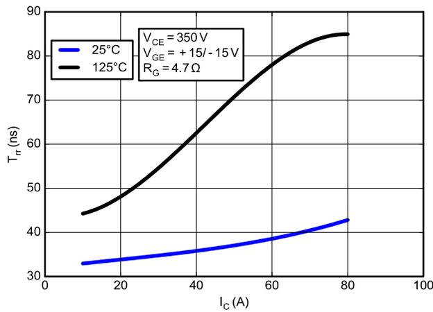
Figure 12. Typical Reverse Recovery Time vs. IC
