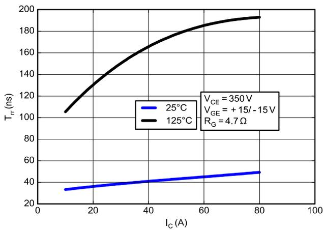
Figure 32. Typical Reverse Recovery Time vs. IC
