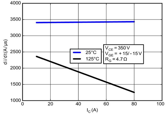
Figure 15. Typical Diode Current Slope vs.  $I_C$
