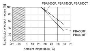
Fig.7.4 Ambient temperature derating curve (-F4)
