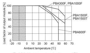
Fig.7.3 Ambient temperature derating curve (-F3)
