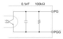
Fig.1.6 Internal circuit of PG
