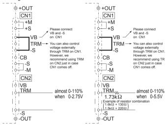
Fig.1.1 Wiring 1
