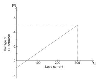
Fig.6.1 Load current conversion graph(PBA1500F-5)
