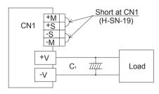
Fig.1.4 When not using remote sensing function
