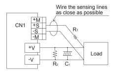
Fig.1.5 When using remote sensing function
