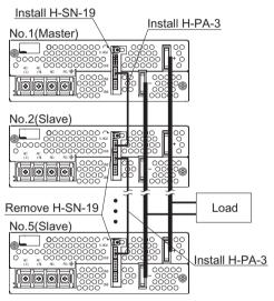
Fig.3.3 Example of parallel connection (PBA1500F)
