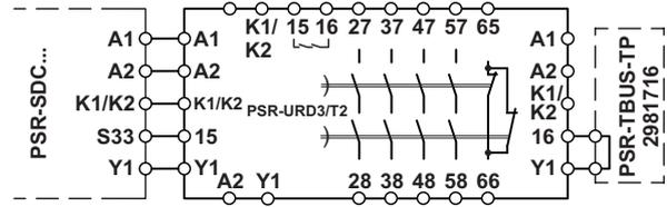
Figure 8 Wiring via T-BUS DIN rail connector
