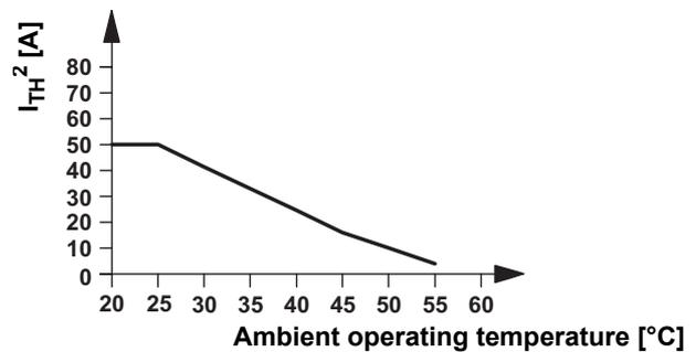
Figure 2 Derating curve
