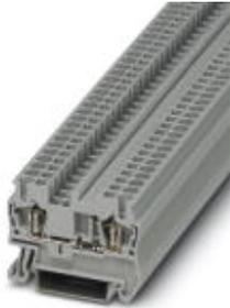
Feed-through terminal block, for installing components that can be individually selected, Connection method: Spring-cage connection, Cross section: 0.08 mm<sup>2</sup> - 4 mm<sup>2</sup>, AWG: 28 - 12, Width: 5.2 mm, Color: gray, Mounting type: NS 35/7,5, NS 35/15
