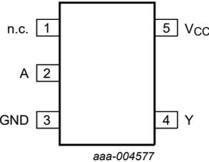
**Fig. 4. Pin configuration SOT353-1 (TSSOP5) and SOT753 (SC-74A)**
