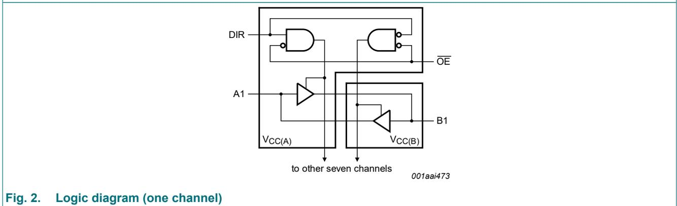
Fig. 2. Logic diagram (one channel)
