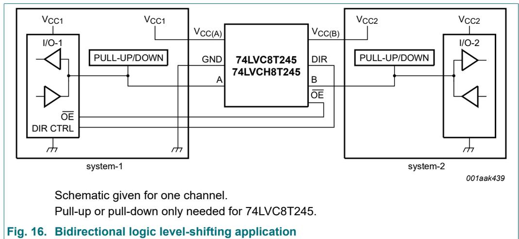
Fig. 16. Bidirectional logic level-shifting application
