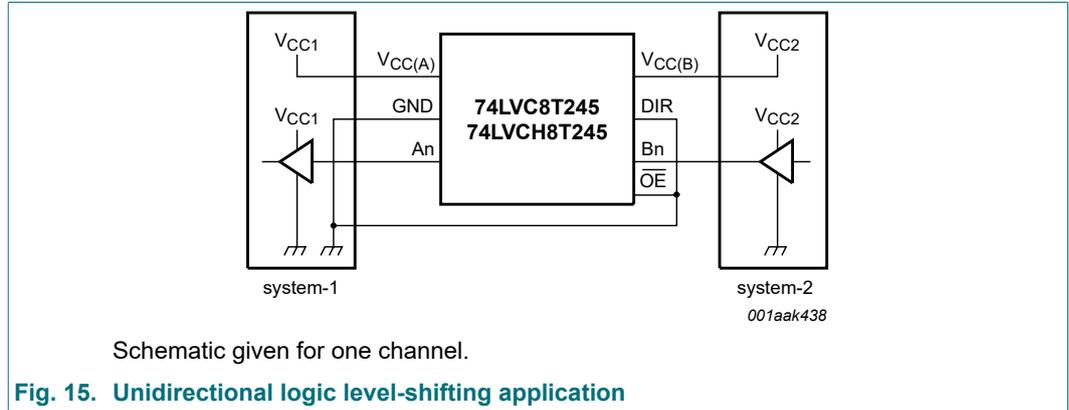
Fig. 15. Unidirectional logic level-shifting application
