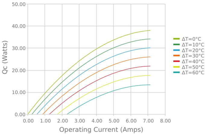
Heat Pumped at Cold Side
