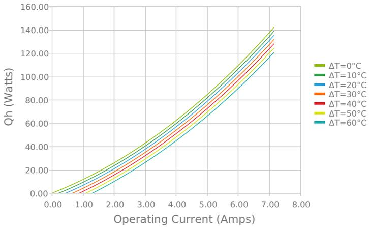
Total Heat Dissipated at Hot Side (Qh=Qc+Pin)
