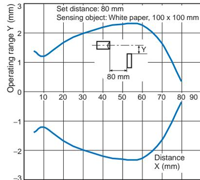
Spot Diameter vs. Sensing Distance
