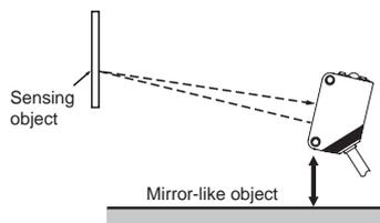
• Do not install the Sensor in the wrong direction. Refer to the following illustration.
