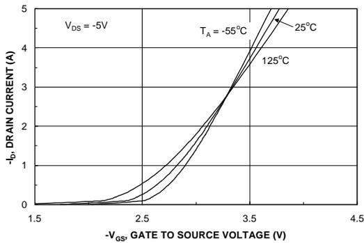
Figure 15. Transfer Characteristics.
