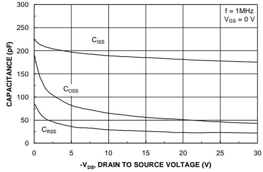
**Figure 18. Capacitance Characteristics.**
