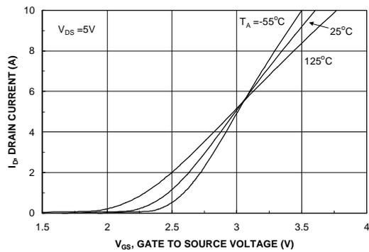
Figure 5. Transfer Characteristics.
