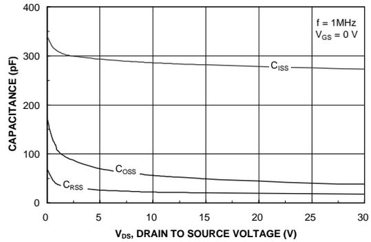
**Figure 8. Capacitance Characteristics.**
