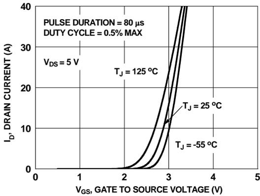
Figure 5. Transfer Characteristics
