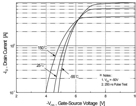
Figure 2. Transfer Characteristics
