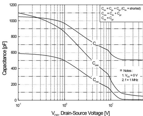
Figure 5. Capacitance Characteristics
