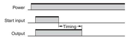
\* The start input is valid while the Timer is in operation.
