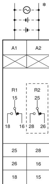
\* The power supply terminals do not have polarity.
