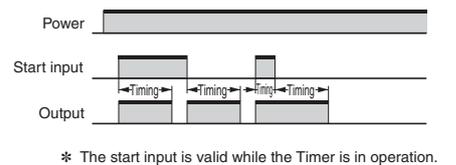
**Note:** 1. The reset time is 0.1 s min. Make sure the signal input time is 0.05 s or longer.
