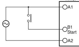
Operates when relay turns ON.
