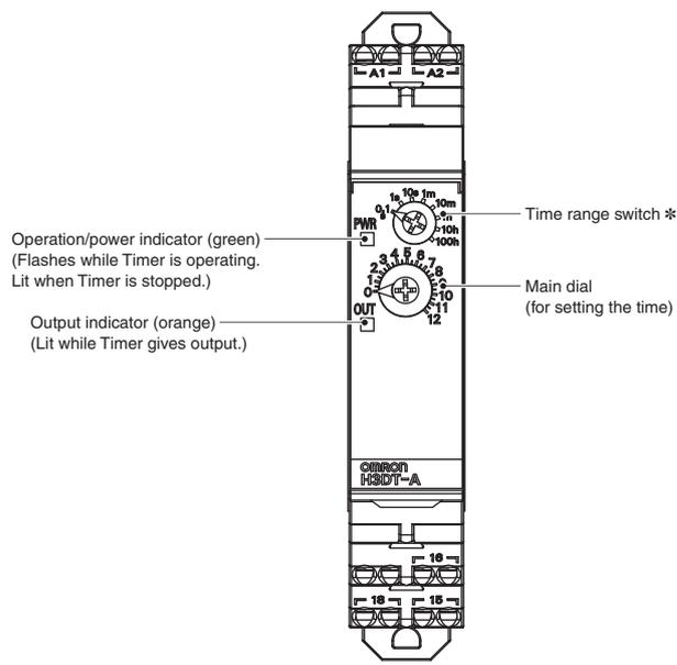
\* If the switch is left between settings, proper operation may not be possible.
