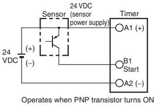
Operates when PNP transistor turns ON.
