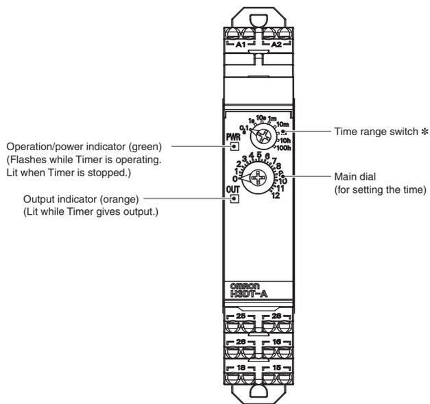
\* If the switch is left between settings, proper operation may not be possible.
