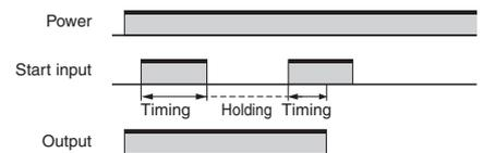
Note: Timing is performed while the start input is ON.
