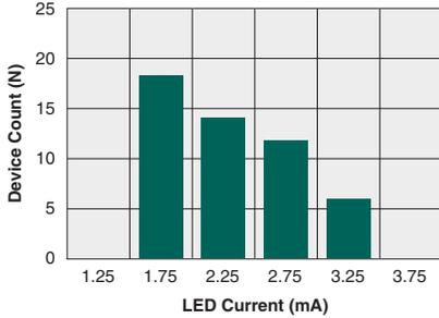
**Typical I<sub>F</sub> for Switch Dropout**
