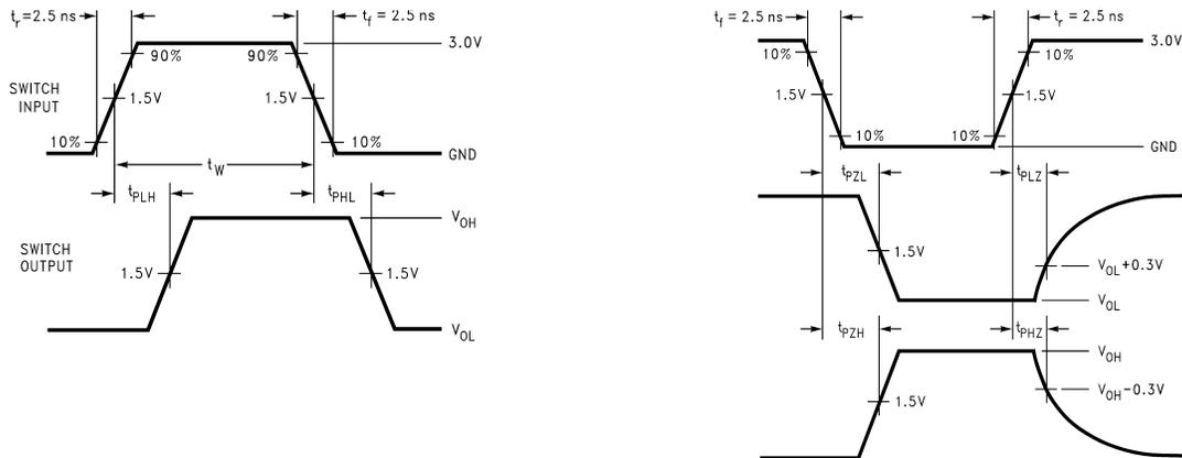
FIGURE 2. AC Waveforms
