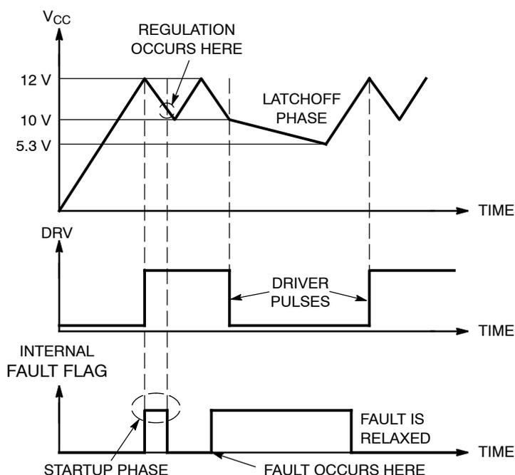
If the fault is relaxed during the V<sub>CC</sub> natural fall down sequence, the IC automatically resumes. If the fault still persists when V<sub>CC</sub> reached V<sub>CCON</sub>, then the controller cuts everything off until recovery.
