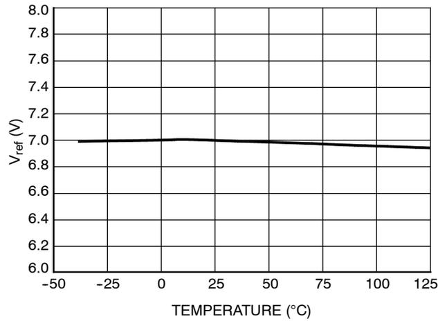
**Figure 11. OVP internal Reference Level versus Temperature**
