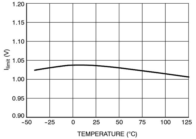
**Figure 10. Maximum Internal Current Setpoint versus Temperature**
