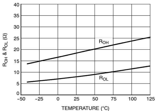
**Figure 8. Source and Sink Resistance versus Temperature**
