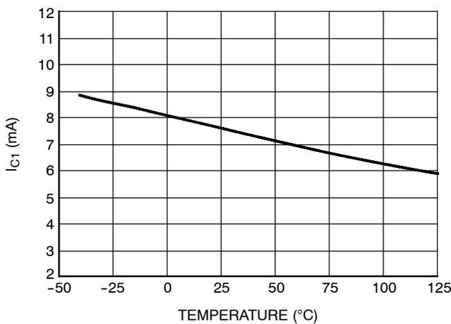
**Figure 7. Internal Startup Current Source at V<sub>CC</sub> = 10 V versus Temperature**
