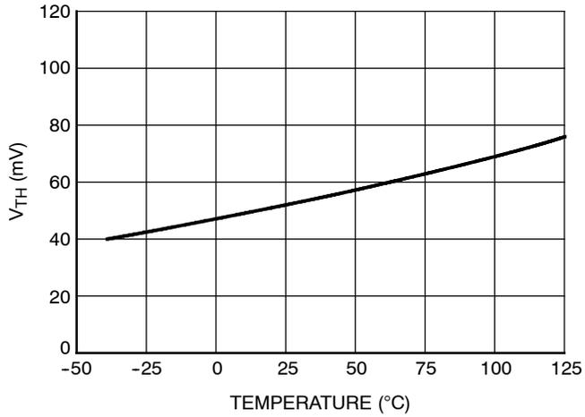
**Figure 9. Input Voltage (Vpin1 Decreasing) versus Temperature**
