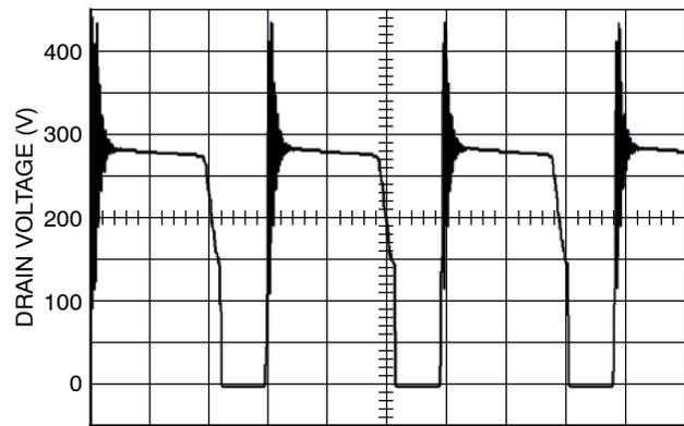
Figure 19. The NCP1207A Operates in Borderline / Critical Operation
