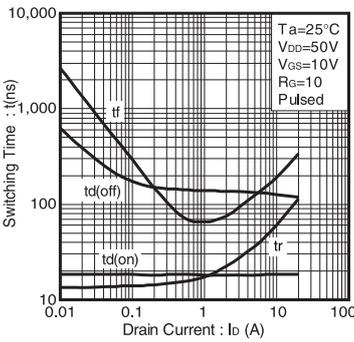
Fig.4 Switching Characteristics
