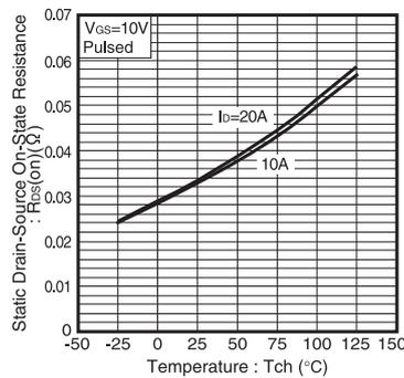
Fig.5 Static Drain-Source On-State Resistance vs. Channel Temperature
