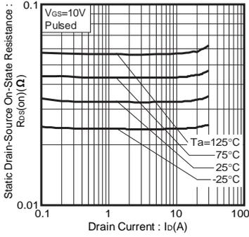
Fig.1 Static Drain-Source On-State Resistance vs. Drain Current
