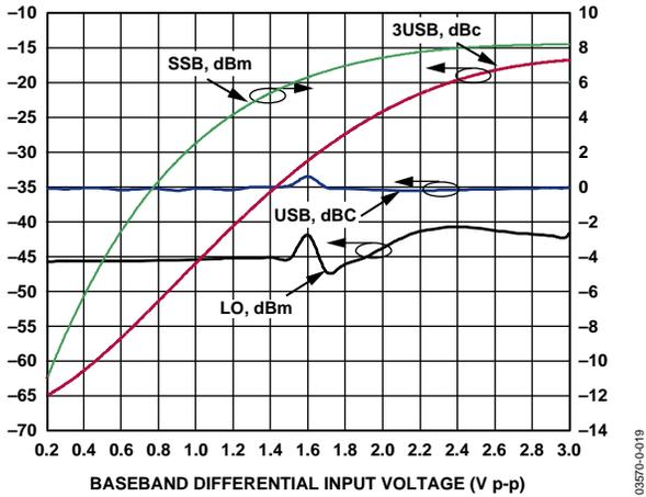
Figure 19. Third Order Distortion (3USB), Carrier Feedthrough, Sideband Suppression, and SSB  $P_{OUT}$  vs. Baseband Differential Input Level ( $F_{LO} = 900$  MHz,  $F_{BB} = 1$  MHz, I and Q Inputs Driven in Quadrature,  $T_A = 25^\circ\text{C}$ )
