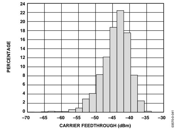
Figure 39. Carrier Feedthrough Distribution at  $F_{LO} = 2140\text{ MHz}$  ( $F_{BB} = 1\text{ MHz}$ ,  $I$  and  $Q$  Inputs Driven in Quadrature at  $1.2\text{ V}_{p-p}$ ,  $T_A = 25^\circ\text{C}$ )
