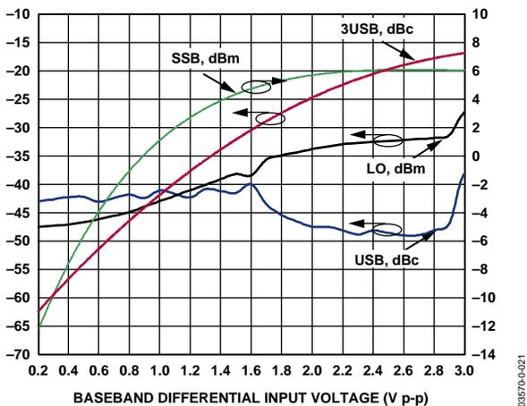
Figure 21. Third Order Distortion (3USB), Carrier Feedthrough, Sideband Suppression, and SSB  $P_{OUT}$  vs. Baseband Differential Input Level ( $F_{LO} = 2140$  MHz,  $F_{BB} = 1$  MHz, I and Q Inputs Driven in Quadrature,  $T_A = 25^\circ\text{C}$ )
