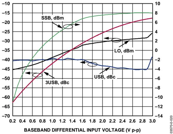
Figure 20. Third Order Distortion (3USB), Carrier Feedthrough, Sideband Suppression, and SSB  $P_{OUT}$  vs. Baseband Differential Input Level ( $F_{LO} = 1900$  MHz,  $F_{BB} = 1$  MHz, I and Q Inputs Driven in Quadrature,  $T_A = 25^\circ\text{C}$ )
