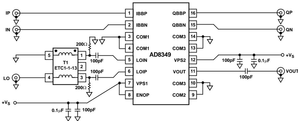
Figure 43. Basic Connections
