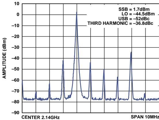
Figure 53. AD8349 Single Sideband Spectrum at 2140 MHz
