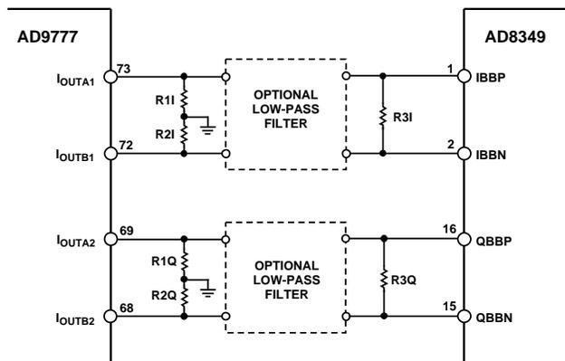
Figure 51. Basic AD9777 to AD8349 Interface
