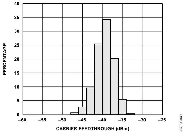
Figure 38. Carrier Feedthrough Distribution at  $F_{LO} = 1900\text{ MHz}$  ( $F_{BB} = 1\text{ MHz}$ ,  $I$  and  $Q$  Inputs Driven in Quadrature at  $1.2\text{ V}_{p-p}$ ,  $T_A = 25^\circ\text{C}$ )
