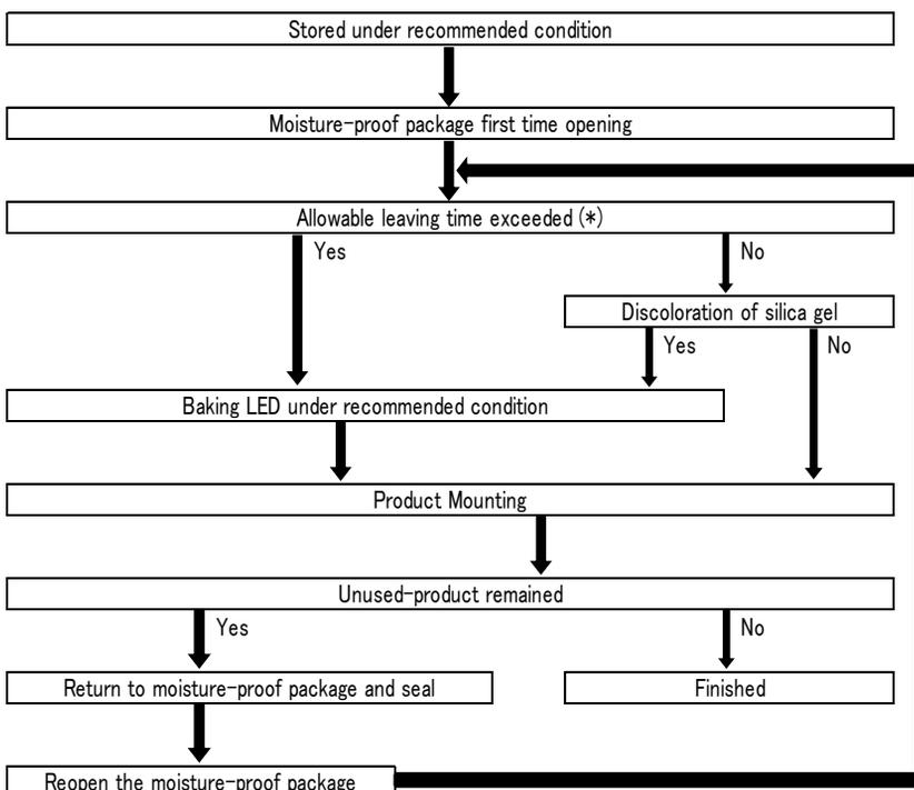
Allowable leaving time means the maximum allowable leaving time after opening package, which depends on each LED type. The allowable leaving time should be calculated from the first opening of package to the time when soldering process is finished. When judging if the allowable leaving time has exceeded or not, please subtract the soldering time. The allowable leaving time after reopening should be calculated from the first opening of package, or from the time when baking process is finished.
