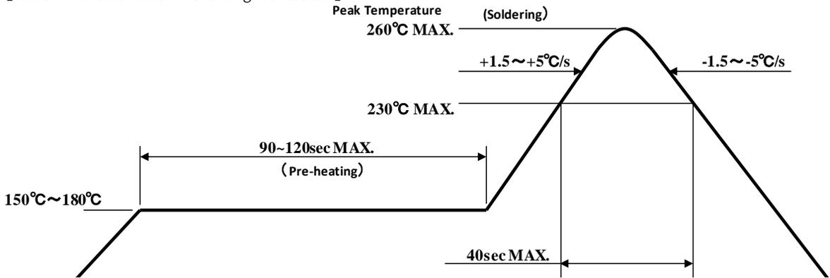
1. The above temp. profile shall be at the surface of LED resin.
