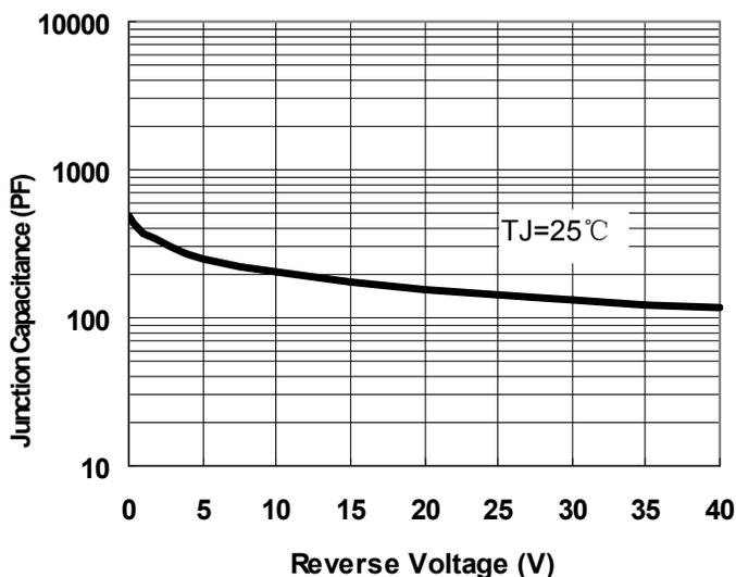
**Fig.1-Typical Junction Capacitance**
