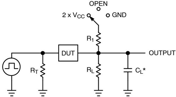
C<sub>L</sub> includes probe and jig capacitance
