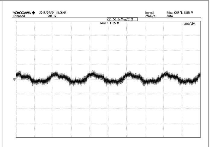
**Figure 6:** Output ripple & noise at 110/220Vac, 21A  $I_{out}$
