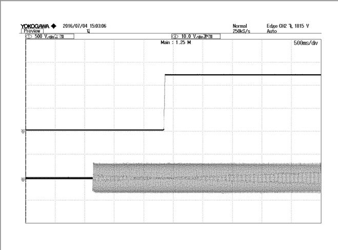
**Figure 5:**  $V_{out}$  start up with Enable on at 220Vac, 21A  $I_{out}$ ,
