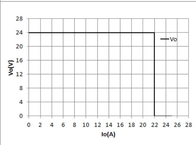
**Figure 3:** Output voltage vs. Output current @  $V_{in}=110/220VAC$
