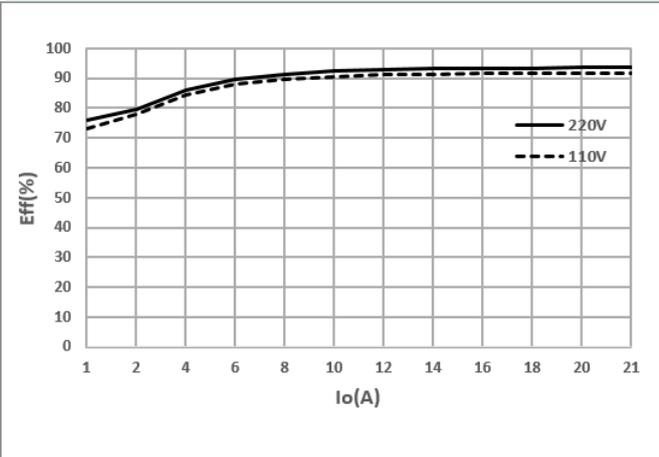
**Figure 1:** Efficiency vs. Output current @  $V_{in}=110,220VAC$
