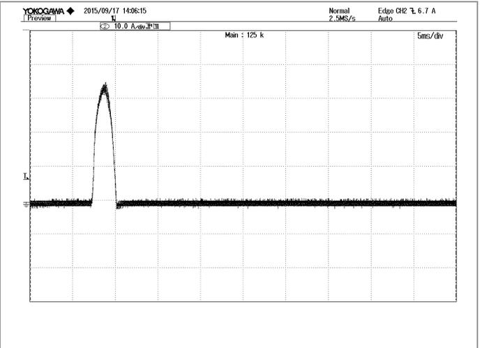
**Figure 8:** Inrush current @ Vin=220Vac lin: 10A/div, 5mS/div;
