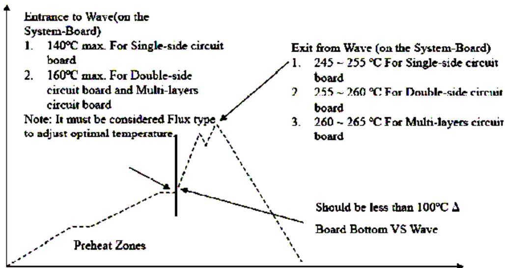
*Note: The temperature is measured on solder joint of pins of power module.*
