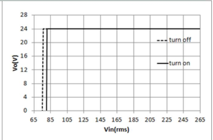
**Figure 2:**  $V_{out}$  vs.  $V_{in}$  @ Full load
