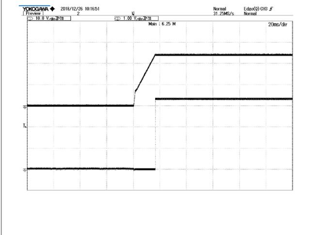
**Figure 9:** PG voltage vs. Vout @ Vin=220Vac, 0Alout
