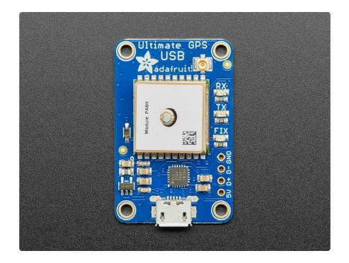
As of March 11, 2022 - we have given this board a makeover! It now comes with a modern USB C connector on the board (instead of micro USB), and a CP2102N instead of CP2104 (functionally-compatible but newer)
