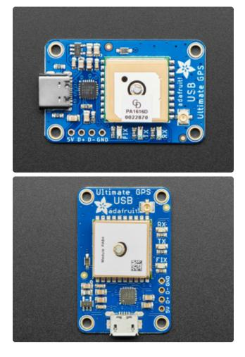
The USB version doesn't have those GPIO pins broken out. Instead it has a single USB serial port. There's 4 pads to the right side that are the USB pinouts for when you want to solder it directly to a USB host controller.
