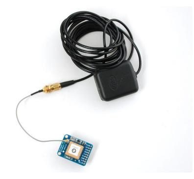
All Ultimate GPS modules have a built in patch antenna - this antenna provides -165 dBm sensitivity and is perfect for many projects. However, if you want to place your project in a box, it might not be possible to have the antenna pointing up, or it might be in a metal shield, or you may need more sensitivity. In these cases, you may want to use an external active antenna. (http://adafru.it/960)
