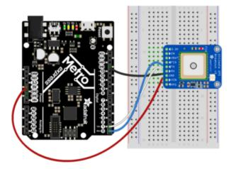
Board 5V or 3.3V to GPS module VIN. Board GND to GPS module GND. Board serial TX to GPS module RX. Board serial RX to GPS module TX.
