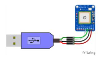
GPS Vin to USB 5V or 3V (red wire on USB console cable) GPS Ground to USB Ground (black wire) GPS RX to USB TX (green wire) GPS TX to USB RX (white wire)
