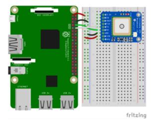
GPS Vin to 3.3V (red wire) GPS Ground to Ground (black wire) GPS RX to TX (green wire) GPS TX to RX (white wire)
