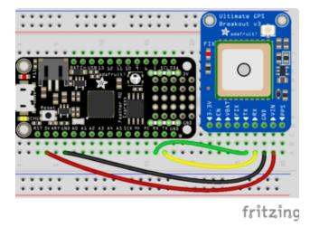
If you're using a board with hardware serial support, like this Feather M0, wire up VIN to 3.3V (since that is the logic level of the Feather M0), GND to ground, and GPS RX to Feather TX and GPS TX to Feather RX.
