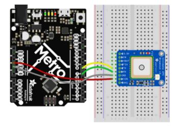
For an Arduino compatible, or any board that does not have an extra HardwareSerial port, we'll use SoftwareSerial. The examples in the Adafruit\_GPS Arduino library use pin 8 for Serial RX and pin 7 for Serial TX on the Arduino-compatible board. The constructor call in the example sketches is SoftwareSerial(8, 7);
