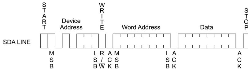
**Page Write:** The 2K EEPROM is capable of an 8-byte Page Write, and the 4K EEPROM device is capable of 16-byte Page Writes.
