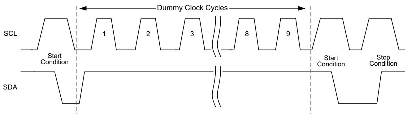
**Figure 6-5. Bus Timing: SCL — Serial Clock, SDA: Serial Data I/O**
