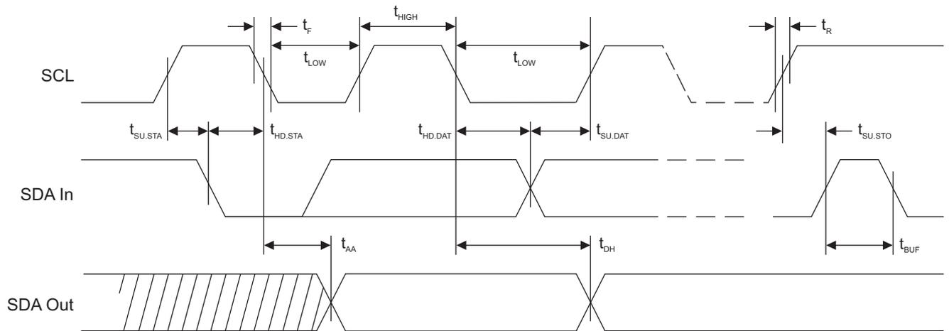
**Figure 6-6. Write Cycle Timing: SCL – Serial Clock, SDA – Serial Data I/O**
