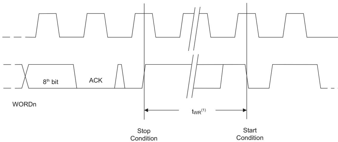
Note: 1. The write cycle time  $t_{WR}$  is the time from a valid Stop condition of a write sequence to the end of the internal clear/write cycle.
