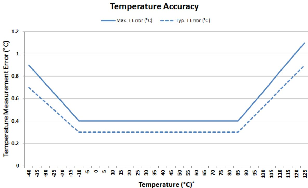
**Figure 3. Temperature Accuracy\***
