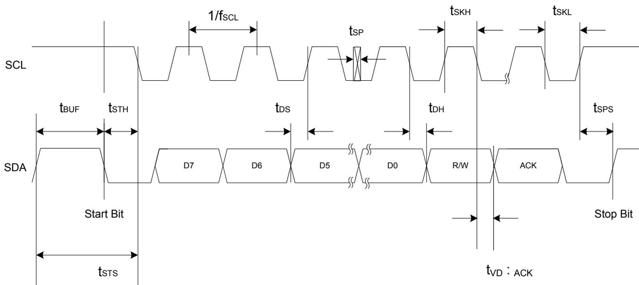
**Figure 1. I<sup>2</sup>C Interface Timing Diagram**
