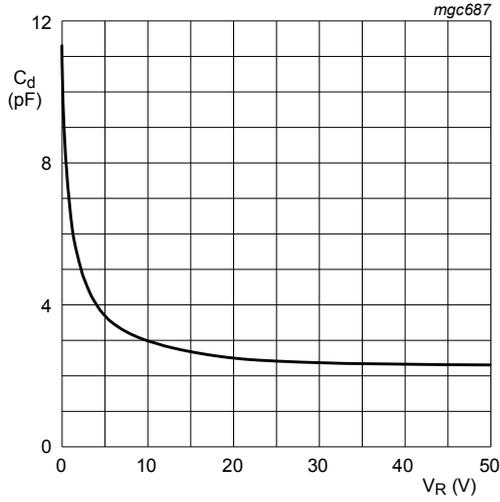
$T_{amb} = 25\text{ °C}; f = 1\text{ MHz}$
