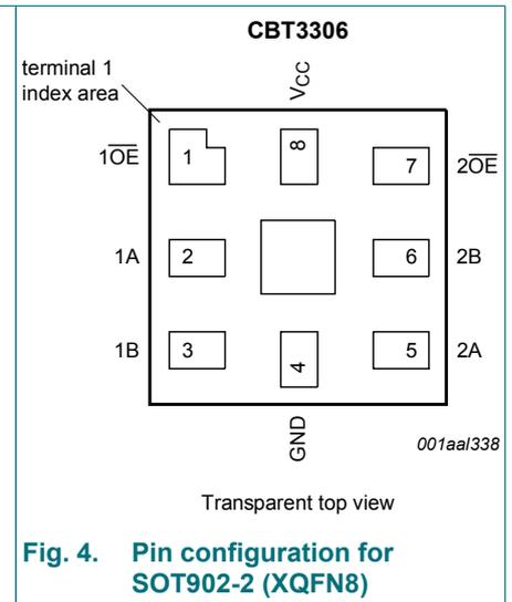
Fig. 4. Pin configuration for SOT902-2 (XQFN8)
