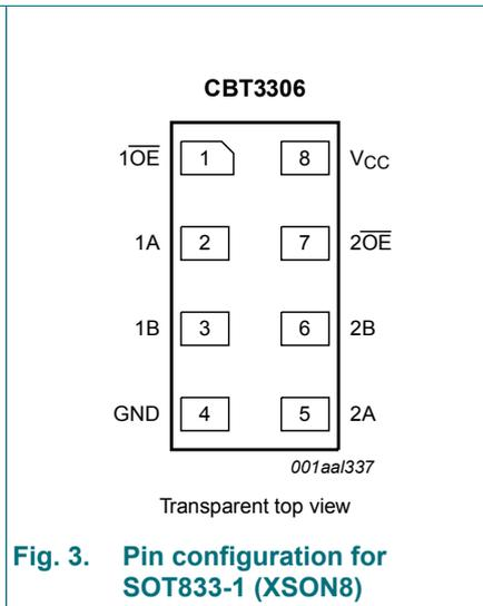
Fig. 3. Pin configuration for SOT833-1 (XSON8)
