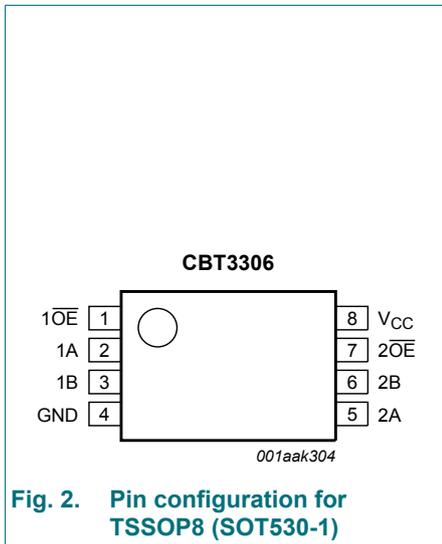
Fig. 2. Pin configuration for TSSOP8 (SOT530-1)
