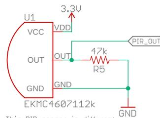
This PIR sensor is different between 170 µA (IC-15368) and 1µA (IC-15370) versions
