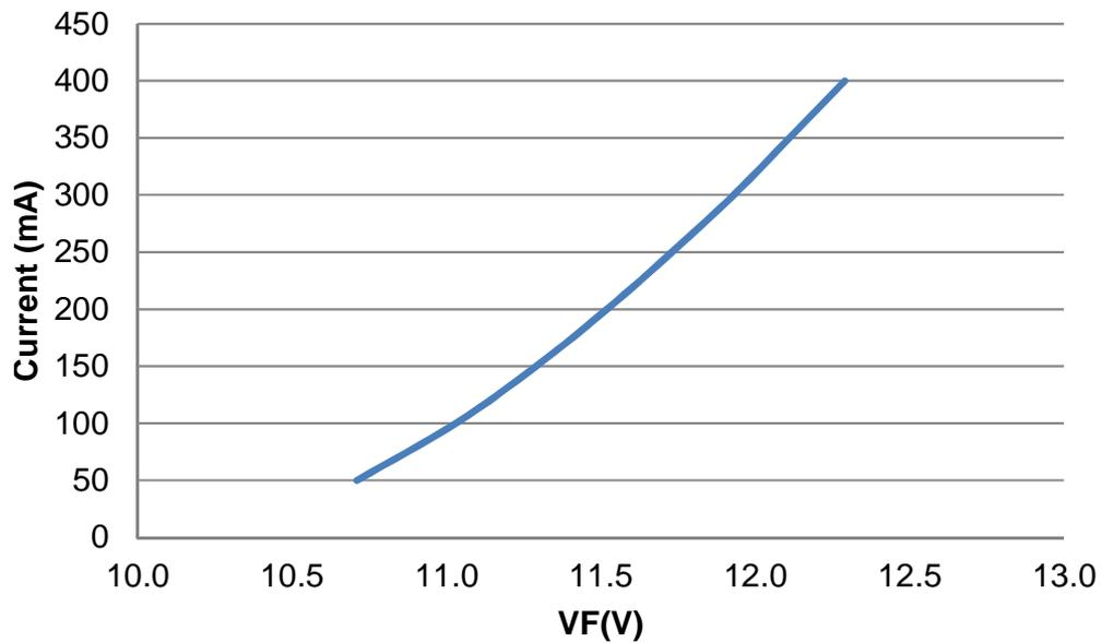
Fig 6. Forward Current vs. Forward Voltage of LTPL-P05EXXXX
