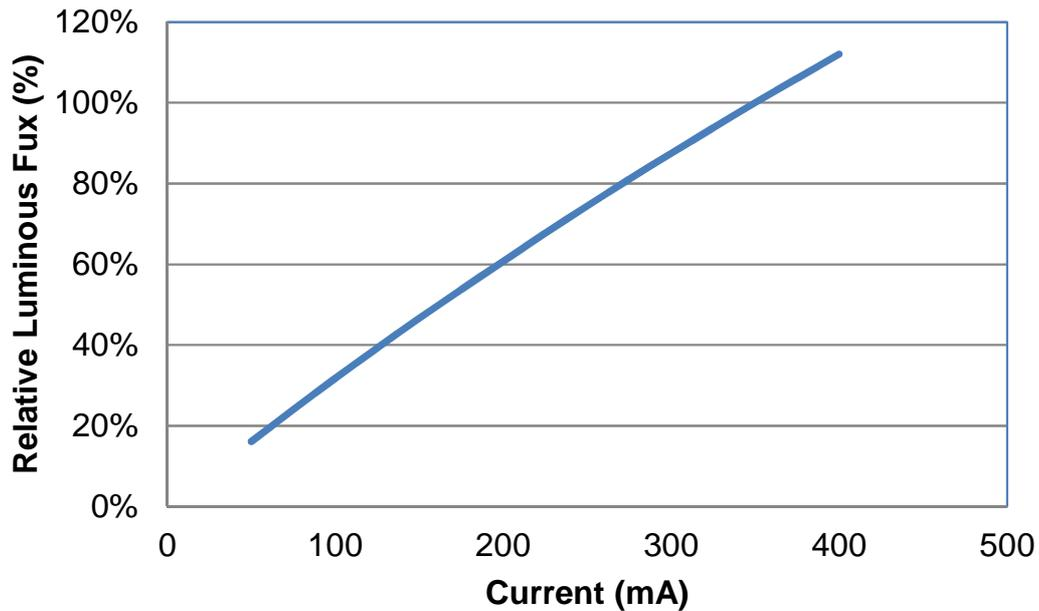
Fig 2. Typical relative luminous flux vs. forward current of LTPL-P05EXXXX
