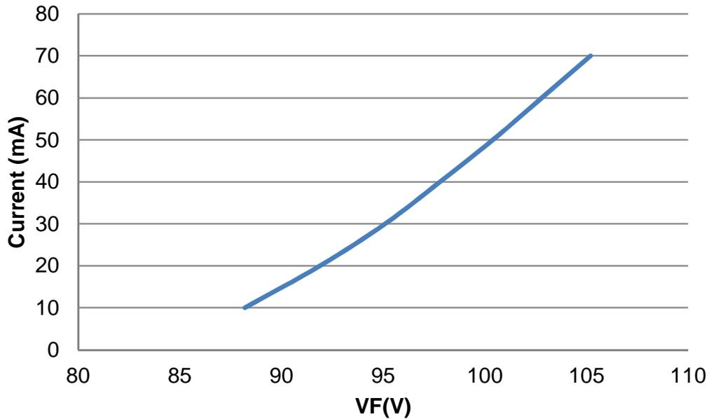
Fig 5. Forward Current vs. Forward Voltage of LTPL-P05DXXXX
