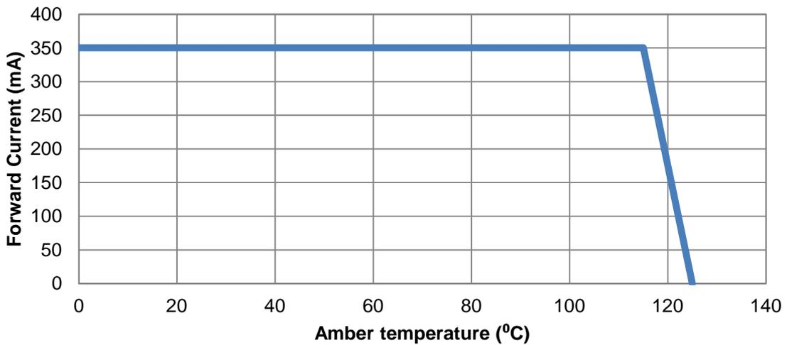
Fig 8. Forward Current Degrading Curve of LTPL-P05EXXXX
