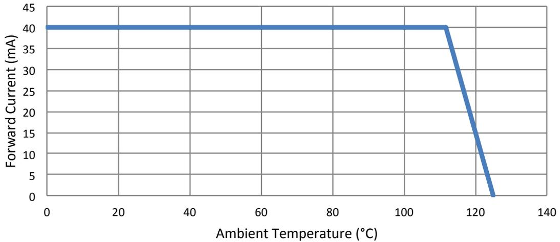
Fig 7. Forward Current Degrading Curve of LTPL-P05DXXXX
