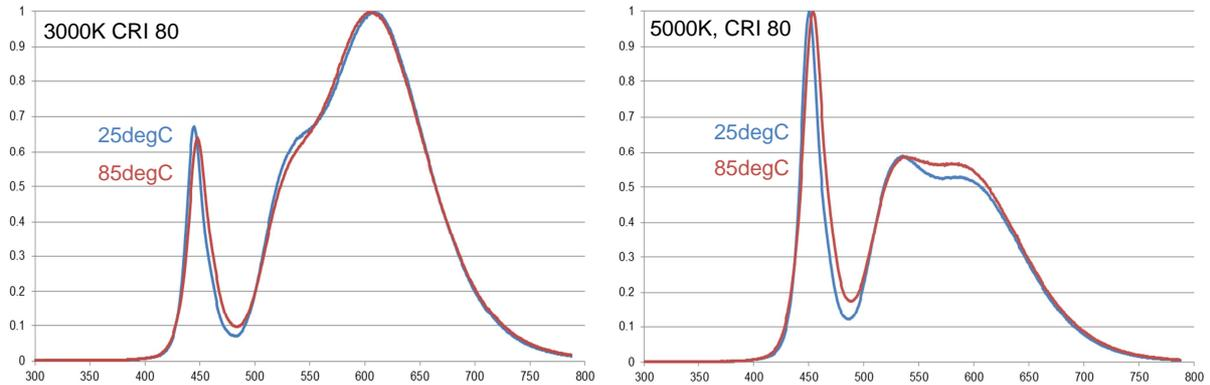
Fig 3. Relative Spectral Distribution at  $T_j = 25^\circ\text{C}$  &  $85^\circ\text{C}$
