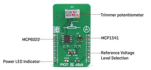
The design uses the MCP6022, a dual, rail-to-rail operational amplifier from Microchip. This operational amplifier is a perfect choice for this design, as it allows rail-to-rail operation, uses a single power supply of 5V, and has a stable unity gain. Without the buffers, the variable impedance would affect the reference voltage. The reference voltage IC can provide less than 10 mA, with the significant voltage drop for output currents exceeding 2 mA.
