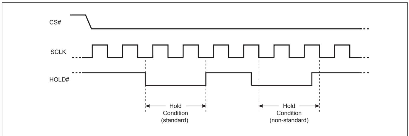
The Serial Data Output (SO) is high impedance, both Serial Data Input (SI) and Serial Clock (SCLK) are don't care during the HOLD operation. If Chip Select (CS#) drives high during HOLD operation, it will reset the internal logic of the device. To re-start communication with chip, the HOLD# must be at high and CS# must be at low.
