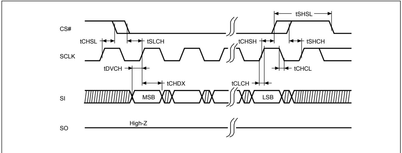
Figure 8. Output Timing
