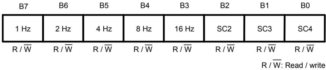
**Figure 15 INT1 Register (Data Register for Output Frequency)**
