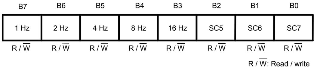
**Figure 16 INT2 Register (Data Register for Output Frequency)**
