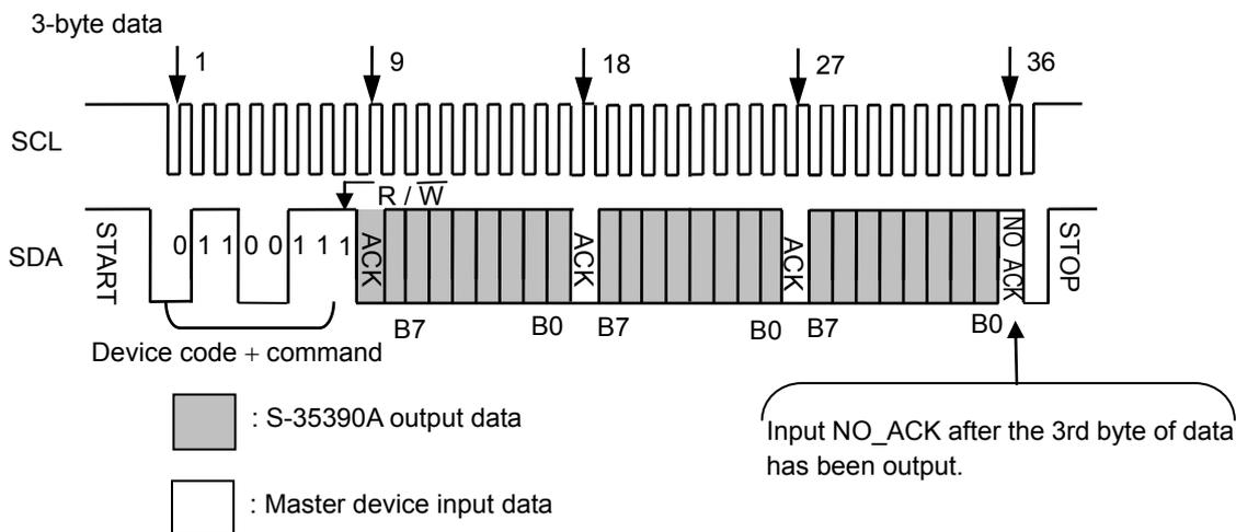
**Figure 36 Example of Data Reading 2 (3-Byte Data Register)**
