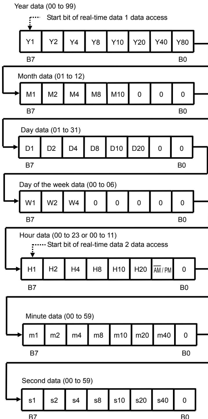
Figure 11 Real-Time Data Register
