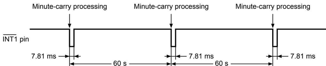
**(2) During reading operation in the real-time data register**
