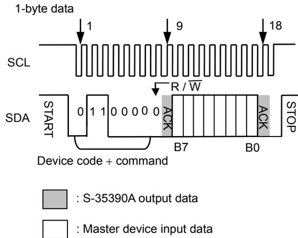
**Figure 37 Example of Data Writing 1 (1-Byte Data Register)**
