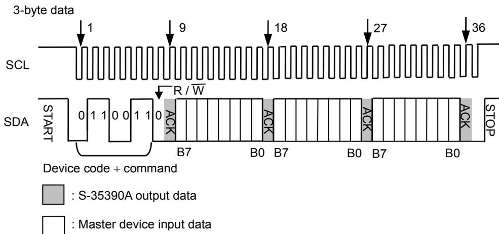
**Figure 38 Example of Data Reading 2 (3-Byte Data Register)**
