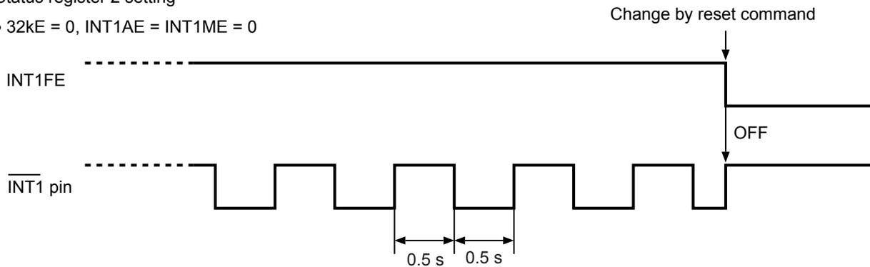
**Figure 31 Output Timing of  $\overline{\text{INT1}}$  Pin during Operation of Power-on Detection Circuit**
