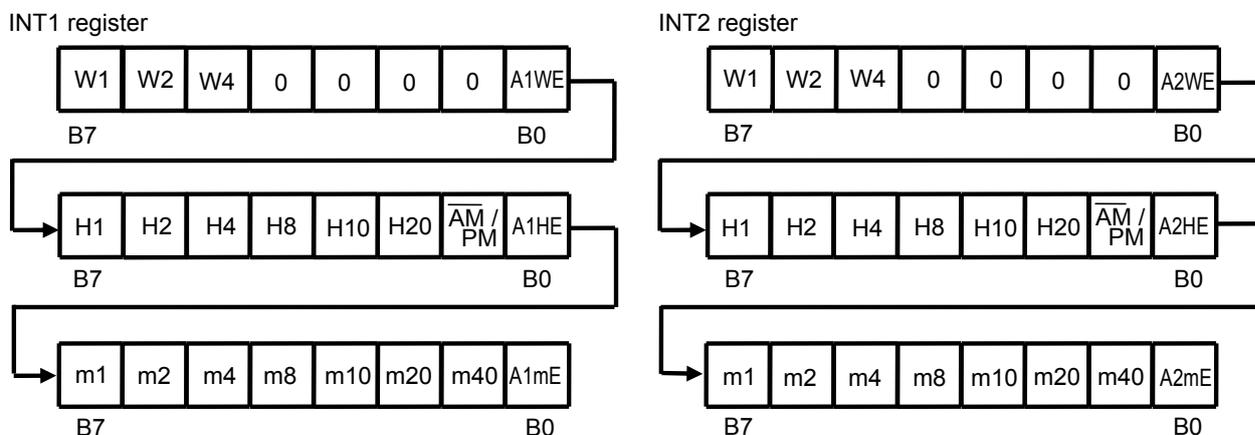
**Figure 14 INT1 Register and INT2 Register (Alarm-Time Data)**
