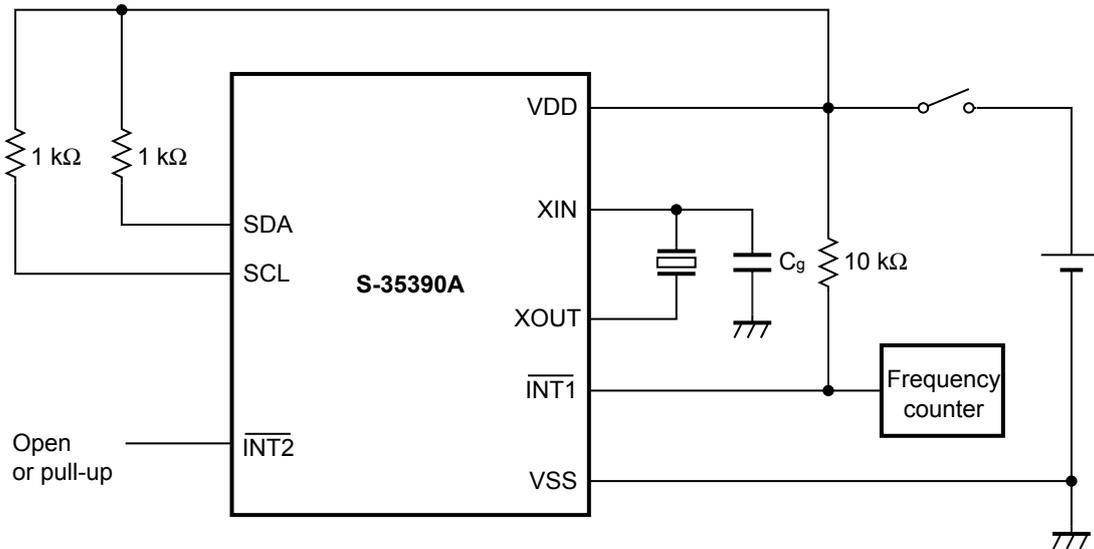
**Figure 52 Configuration of Oscillation Frequency Measurement Circuit**
