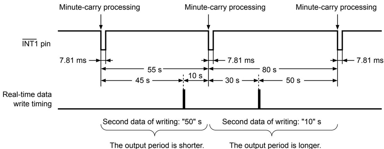
Figure 30 Timing of Minute-periodical Interrupt Output 2
