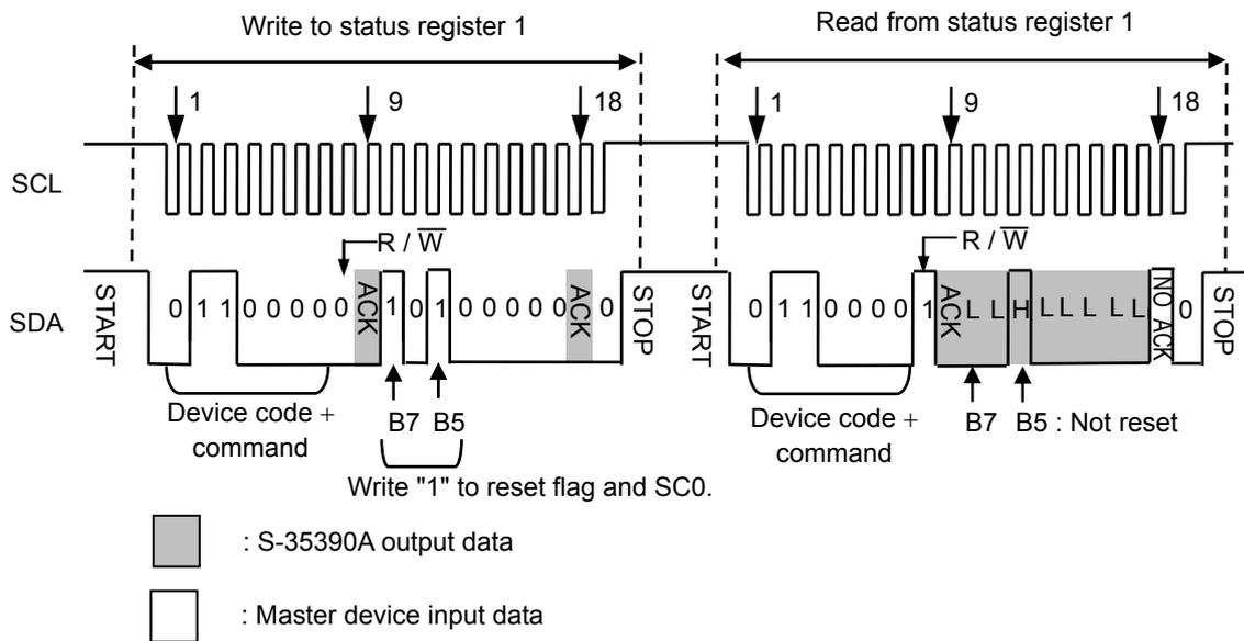
Figure 22 Data of Status Register 1 at Initialization
