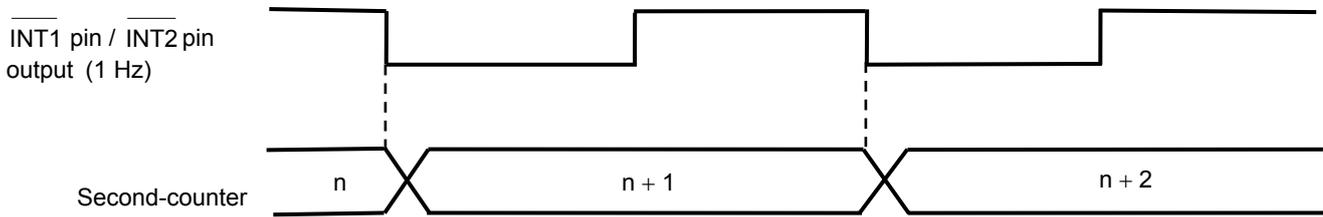
Figure 18 1 Hz Clock Output and Second-counter
