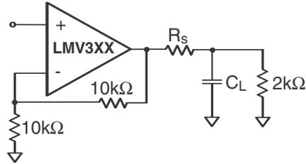
Figure 2. Typical Topology for driving a capacitive load
