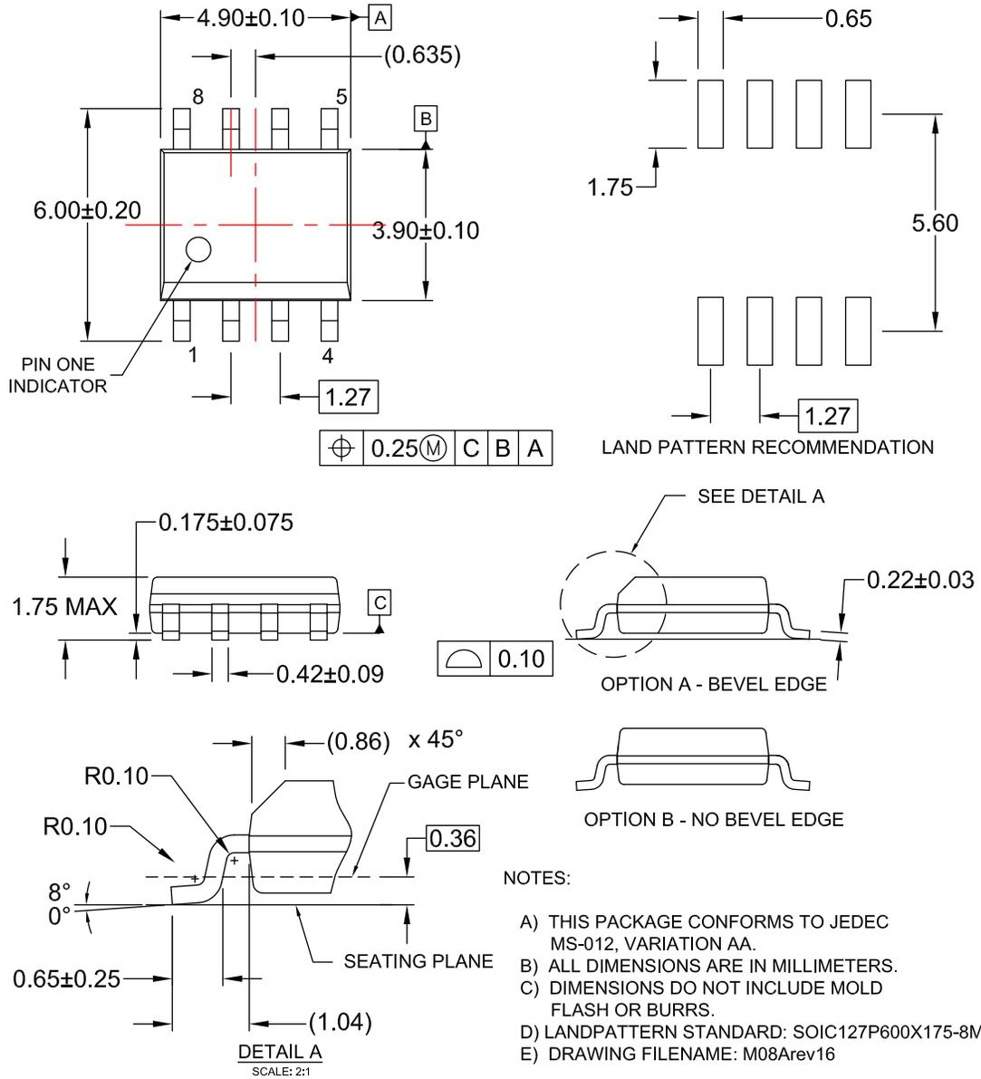
Figure 8. 8-LEAD, SOIC, JEDEC MS-012, 0.150 INCH NARROW BODY
