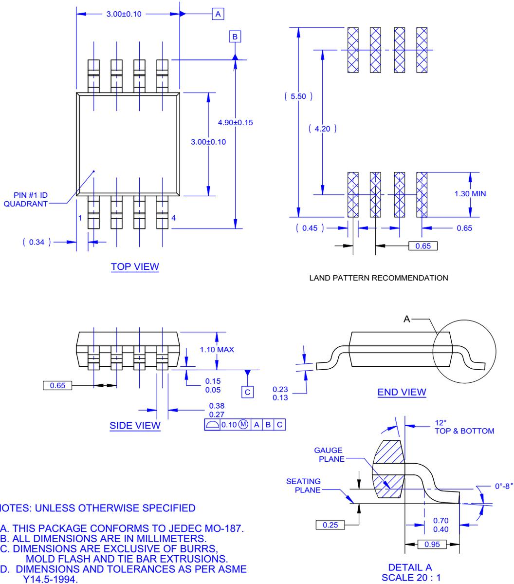
Figure 9. 8-LEAD, MSOP, JEDEC MO-187, 3.0MM WIDE
