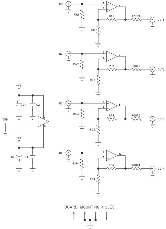
Figure 4d. LMV324 KEB018 schematic
