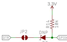
JP2 allow auto-control of GPIO00 for programming. Disconnecting may be required to use serial terminal debugging.
