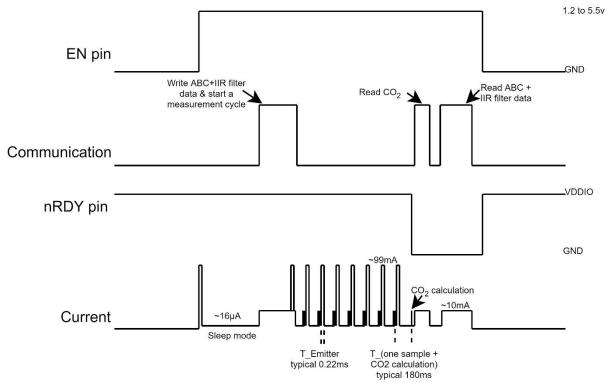
Communication, Timing diagram for single measurement mode
