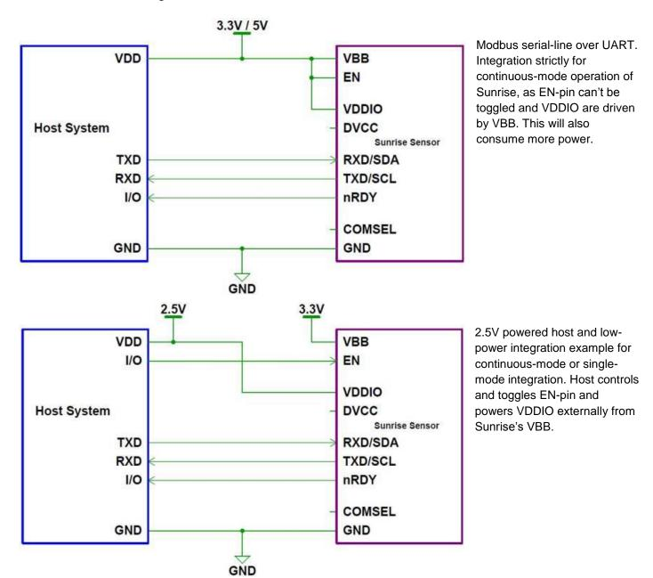
Optionally, although not recommended, an additional GDIO -pin can be saved on host by leaving nRDY floating and implement synchronization and handshaking by worst-case timings.
