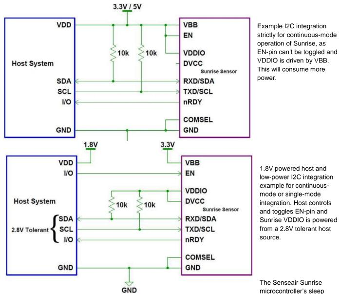
feature, for lower power-consumption between actual memory operations, will wake the device up whenever there's a pulse detected on the SDA-line.
