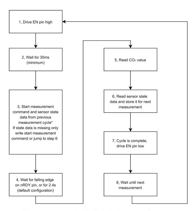
\*If start measurement command and state data is written in two separate write sequences, state data must be written before start measurement command
